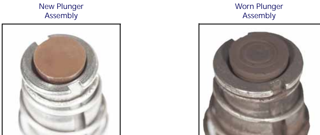
FIGURE 4. Plunger Inspection Detail
