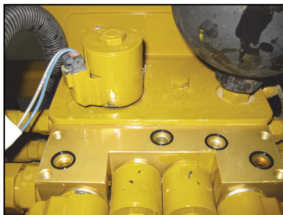
FIGURE 2. O-Rings Placed on the Machine Hydraulic Valve
