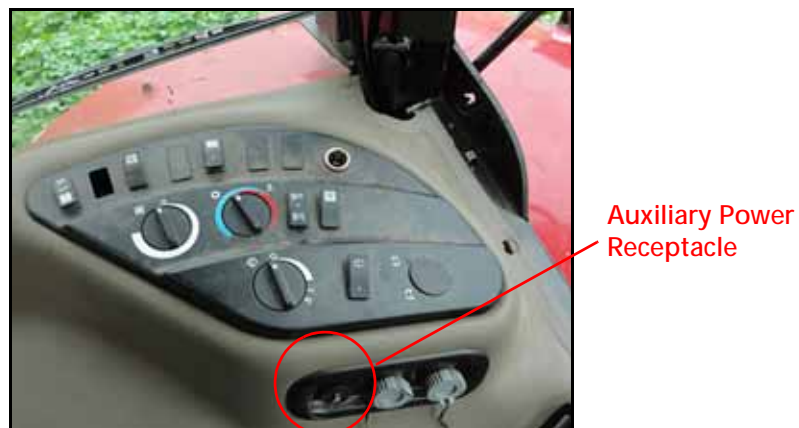
FIGURE 2. Control Panel and Power Panel
