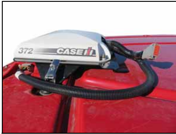
FIGURE 10. GPS Receiver Adapter Cable Connection
