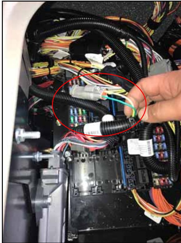
FIGURE 13. ISOBus Extension Harness
