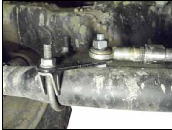
FIGURE 3. Rod End of the WAS Secured to the WAS Bracket
