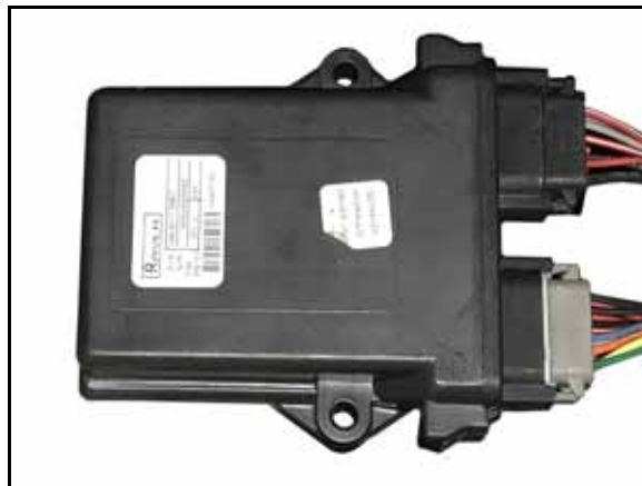
FIGURE 3. SC1/HDU Harness Cable Installed on HDU
