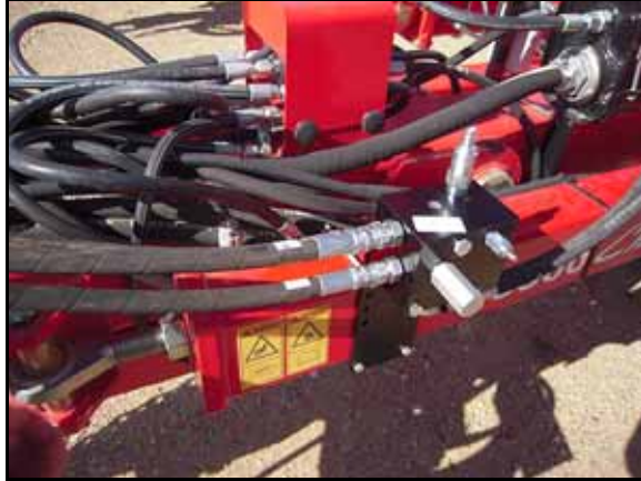
FIGURE 20. OmniRow Valve Pressure and Tank Hoses Installed
