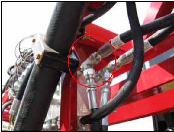
FIGURE 2. Pressure Hoses Installed
