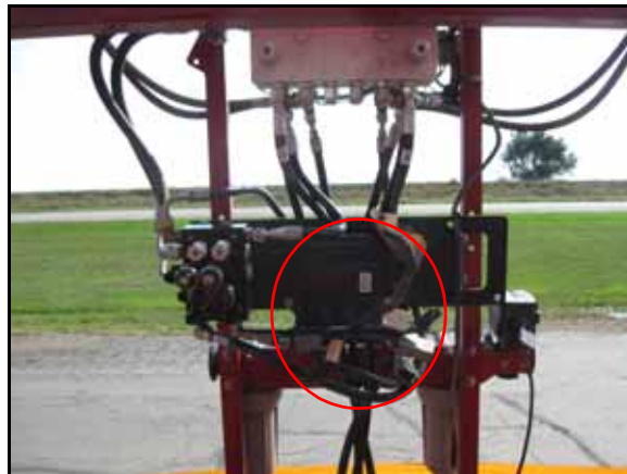
FIGURE 10. AutoBoom Node Installed
