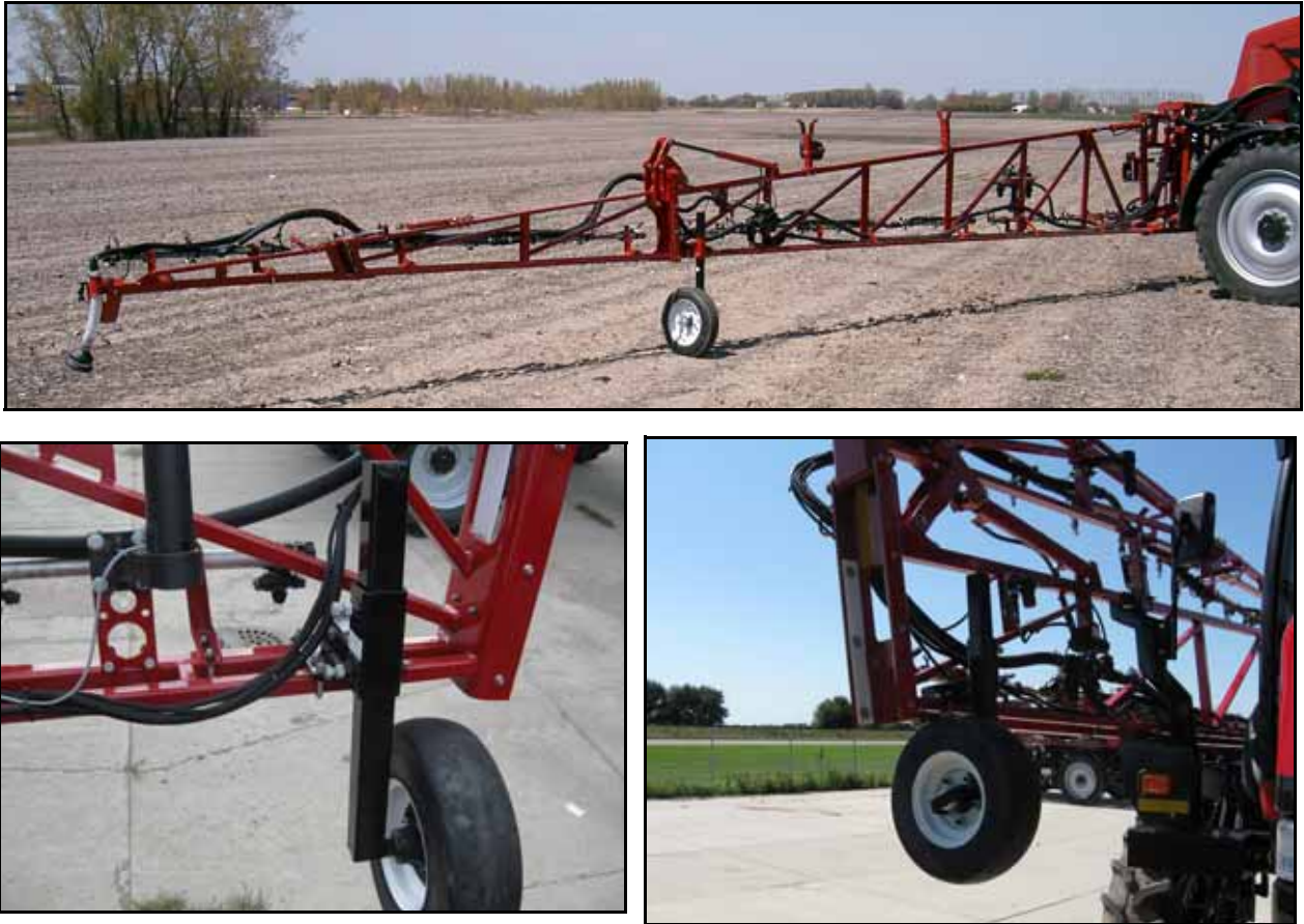
FIGURE 9. Gauge Wheel Installed
