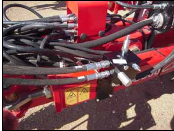
FIGURE 21. OmniRow Valve Pressure and Tank Hoses Installed
