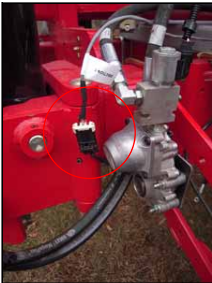
FIGURE 2. Harness Cable Connections on the Row Units
