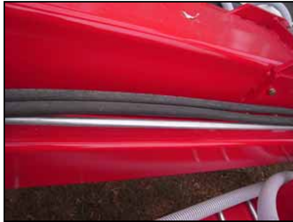
FIGURE 23. Hoses Routed Along Machine's Draw Bar
