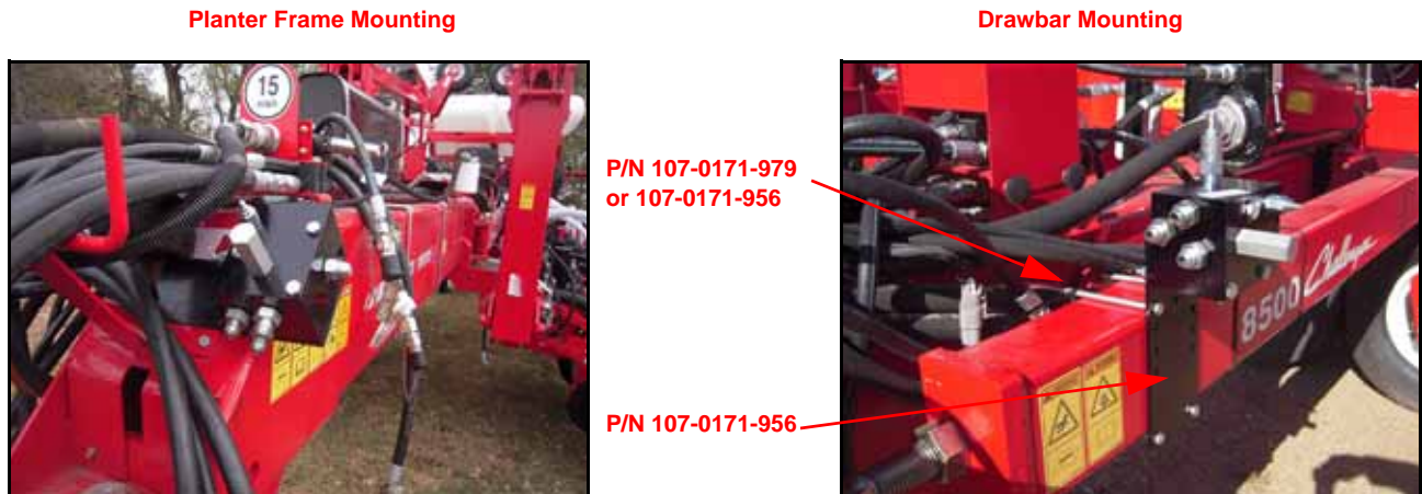
FIGURE 18. OmniRow Hydraulic Valve Installed
