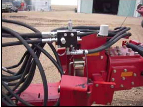
FIGURE 17. OmniRow Valve Pressure and Tank Hoses Installed
