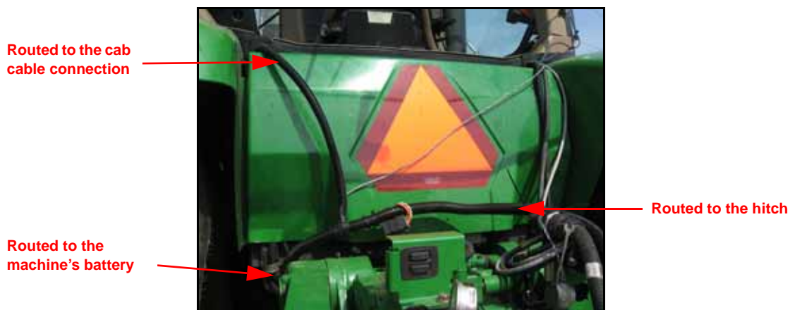
FIGURE 1. Extension Cable Connected to the Tractor Harness Cable
