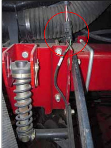
6. Connect the remaining 3-pin weatherpack connector to the installed seed tube sensor on the first row unit.
