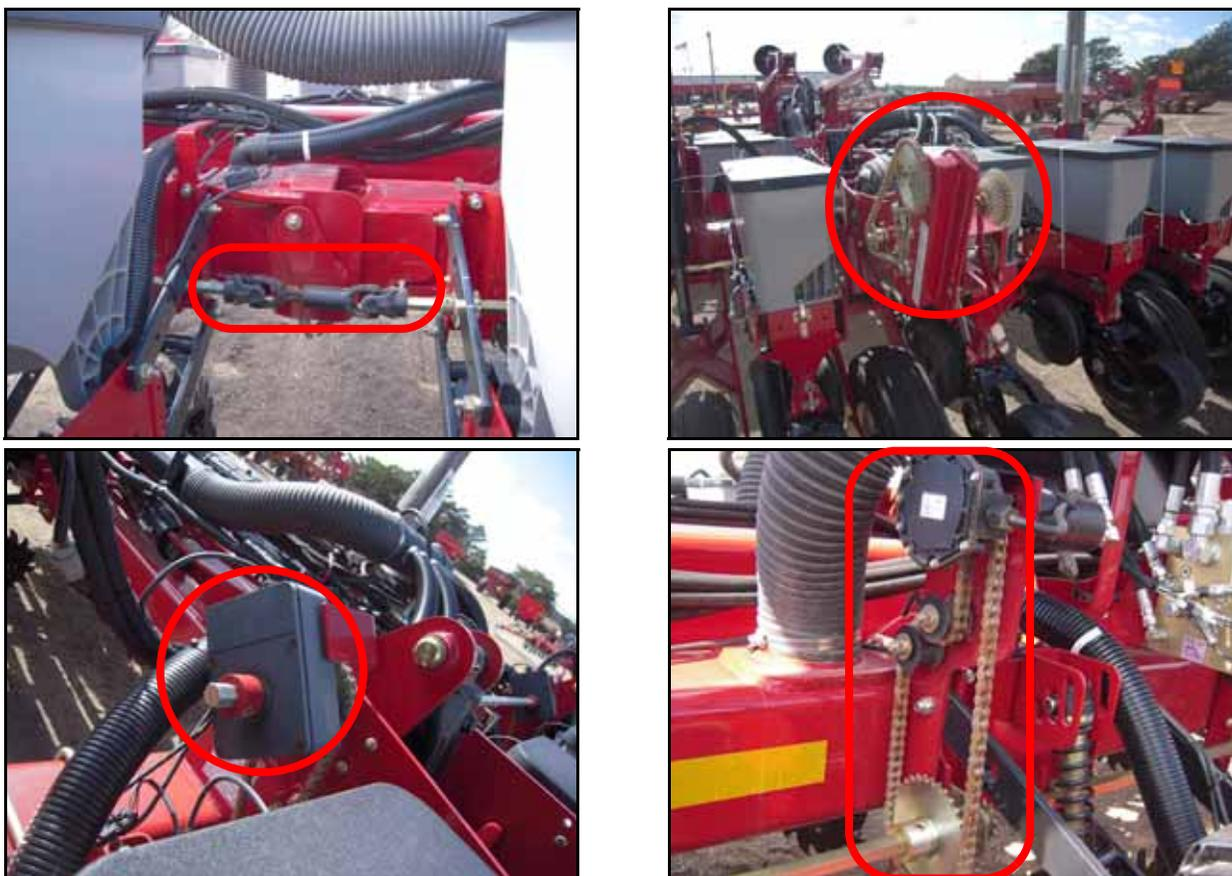
6. Remaining jack shafts, transmissions, and/or OEM hydraulic motors can be removed as needed if they interfere with the OmniRow installation.
