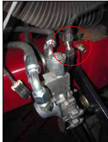
4. Connect the 3-pin metripack connector labeled Section 1 to the motor speed sensor of the hydraulic motor installed on the first row unit.
