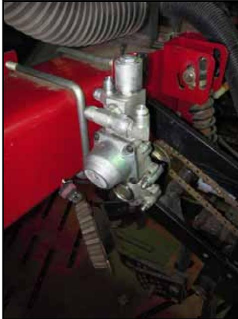
4. Mount the hydraulic motor (P/N 416-8001-001) to the motor mounting bracket using 3/8" x 2-1/2" L bolts (P/N 311-0054-111) and loosely secure with 3/8" zinc flanged lock nuts.
