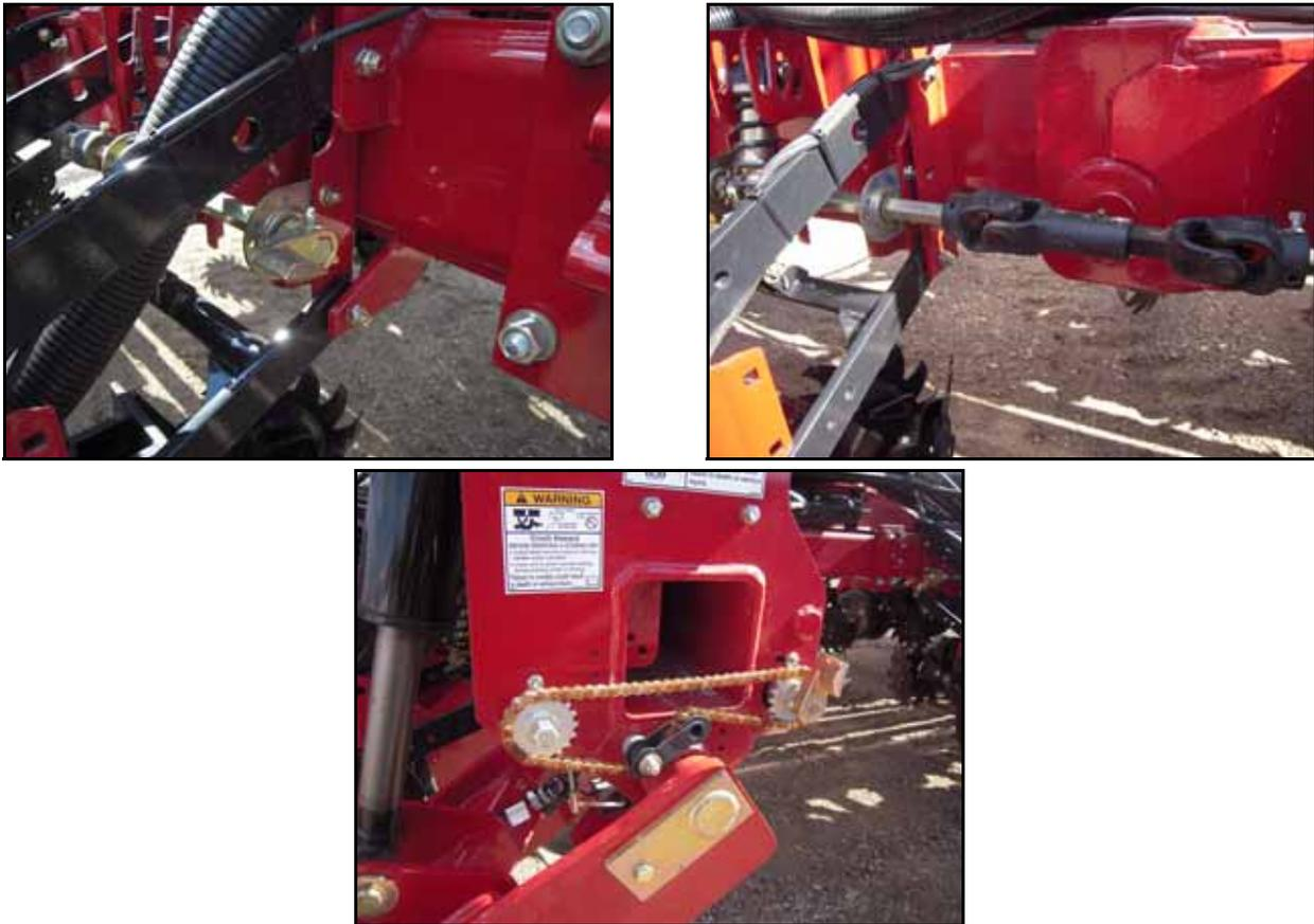
5. Supplemental support bearings (from the right side of the planter row units, opposite the seed meter drive sprocket) can be removed as needed if they interfere with the OmniRow installation.
