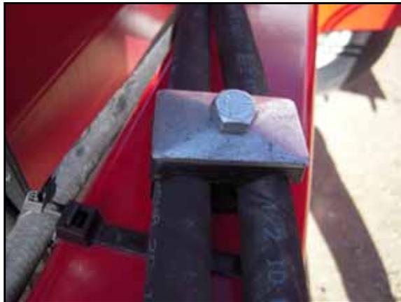
**Note:** Use the provided hose clamps (P/N 434-2000-001) to secure the installed hydraulic lines to each end of the machine's draw bar as illustrated in the figure above.
