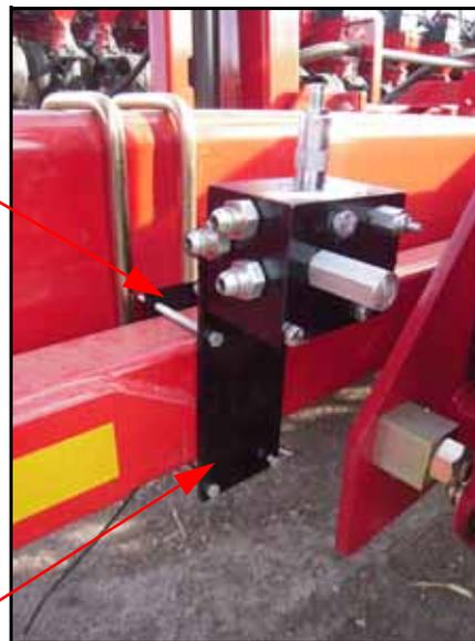
**Note:** The OmniRow hydraulic valve should be mounted at the front of the planter, near the hitch in a location that allows the hydraulic hoses to be connected to it without interference. Refer to the machine-specific hydraulic installation sheet for the location. Ports P, T, and EF should face the planter's hitch and Ports G1, G2, and T2 should face the planter's tool bar if possible.
