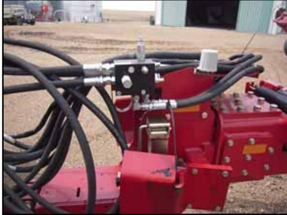
Refer to the supplied machine-specific hydraulic installation sheet included with the OmniRow installation kit to install the OmniRow hydraulic valve pressure and tank hoses.
