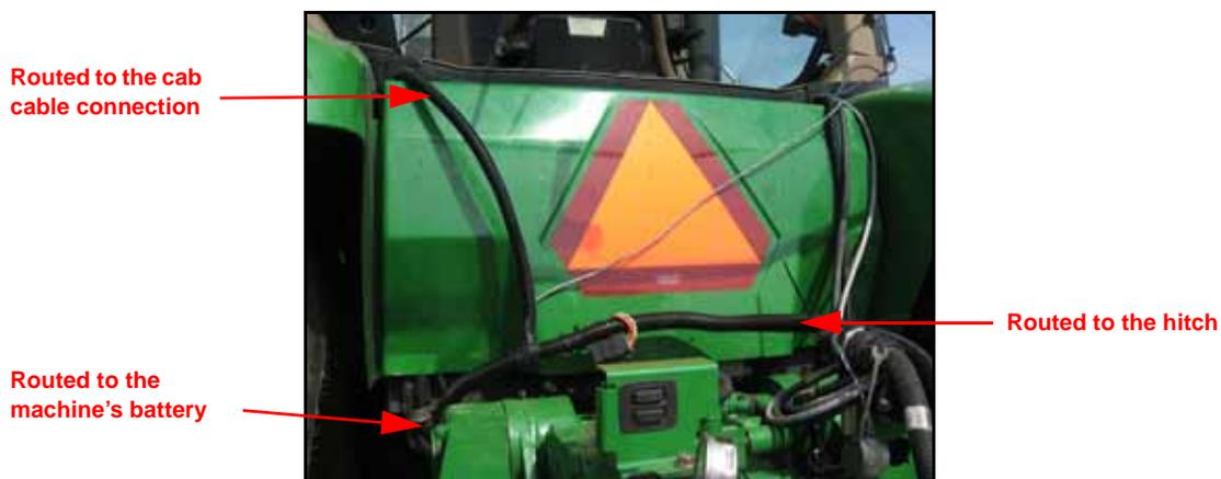
4. Route the cab cable into the cab and connect it to the Envizio Pro II.
