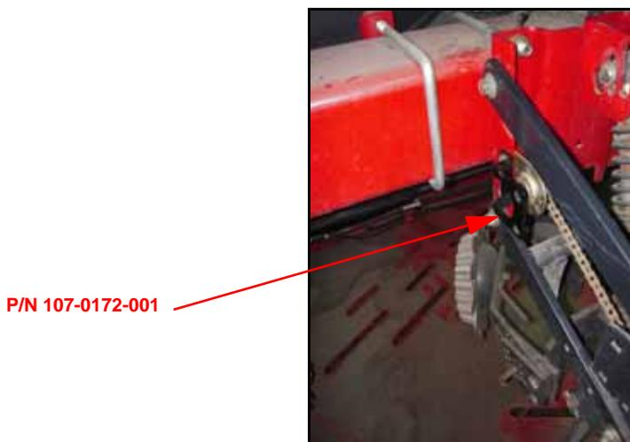
2. Mount the motor mounting bracket (P/N 107-0172-001) on the bolts/studs.
