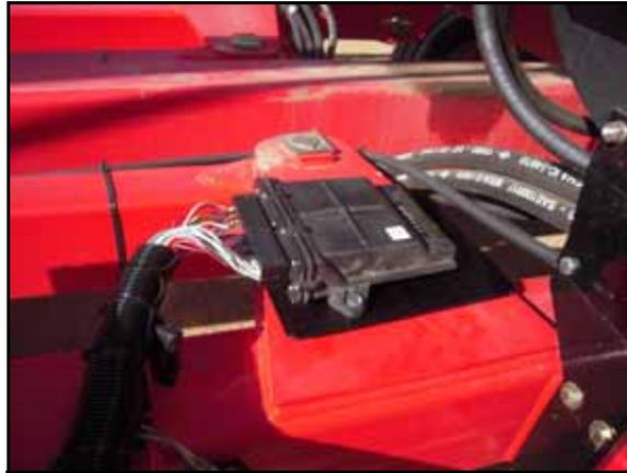
**Note:** The node mounting plate has several options for mounting the magnets. Determine the best node mounting position(s) appropriate for the machine's configuration.
