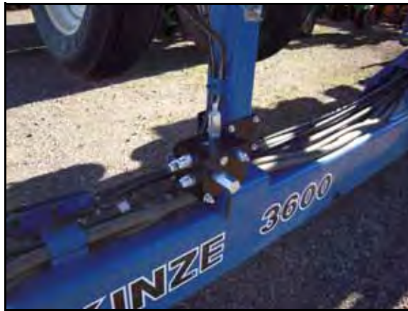
FIGURE 14. Open Center Pressure-Reducing Valve Installed
