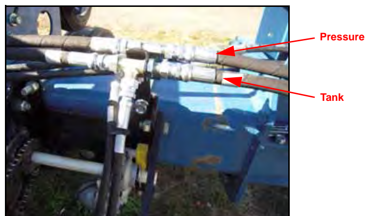
FIGURE 16. Planter Row Unit Pressure and Tank Hoses Installed
