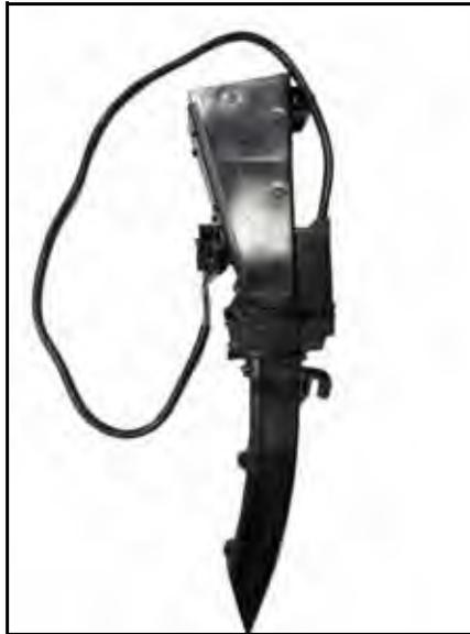
2. Using the supplied cable ties, install the replacement seed tube sensor on the seed tube.
