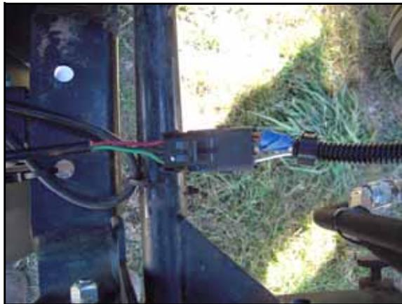
6. Connect the remaining 3-pin weatherpack connector to the installed seed tube sensor on the first row unit.
