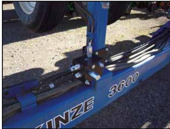
**Note:** The OmniRow hydraulic valve should be mounted at the front of the planter, near the hitch in a location that allows the hydraulic hoses to be connected to it without interference. Refer to the machine-specific hydraulic installation sheet for the location. Ports P, T, and EF should face the planter's hitch and Ports G1, G2, and T2 should face the planter's tool bar if possible.
