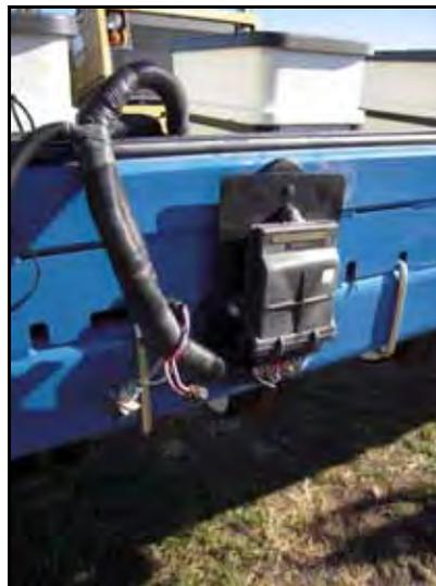
**Note:** *The node mounting plate has several options for mounting the magnets. Determine the best node mounting position(s) appropriate for the machine's configuration.*
