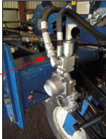
FIGURE 33. Pressure and Tank Hoses Installed - Outboard Mounted Motors
