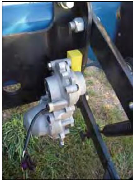
2. Loosely mount the hydraulic motor to the right side of the planter row unit (across from the drive sprocket) using two 3/8"-16 x 7/8" hex socket head cap screws (P/N 311-0068-101).
