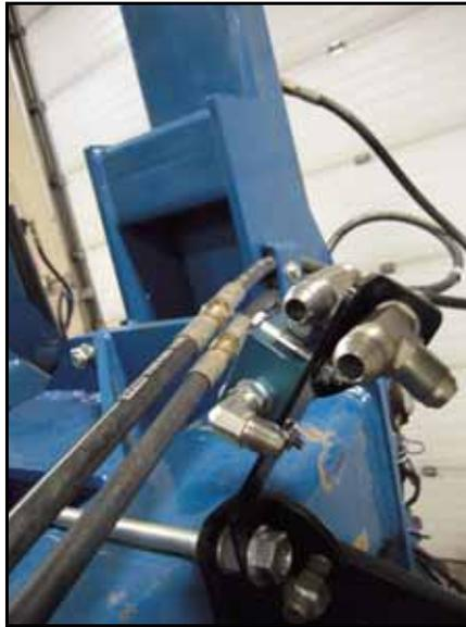
2. Install the PWM valve assemblies on the remaining row units using the supplied 5/8"-11 flanged lock nuts (P/N 312-1001-179).
