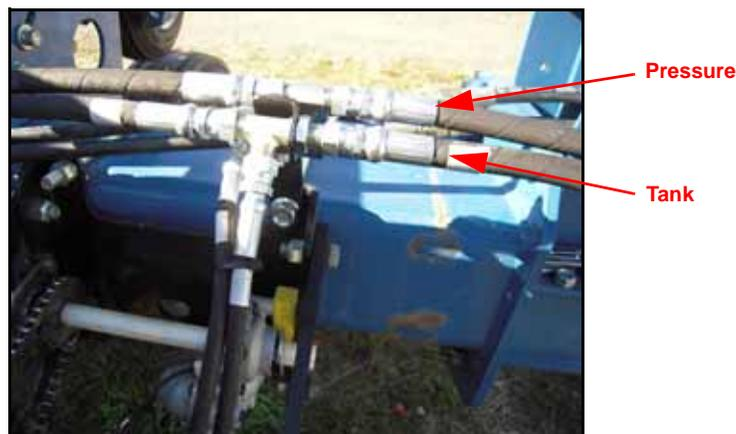
FIGURE 32. Hose Installation Illustration
