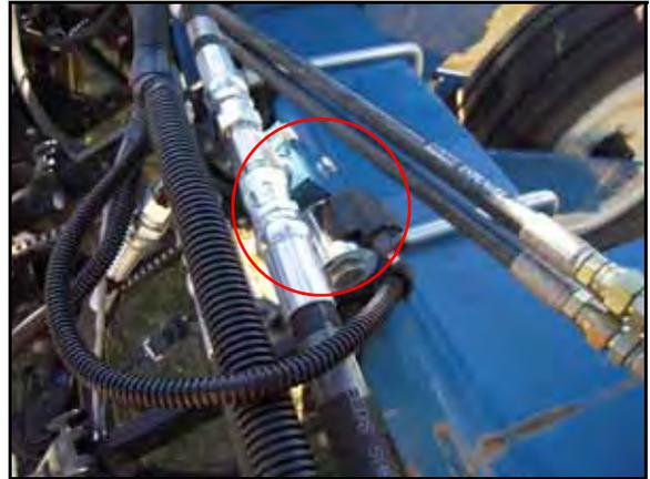
4. Connect the 3-pin metripack connector labeled Section 1 to the motor speed sensor of the hydraulic motor installed on the first row unit.
