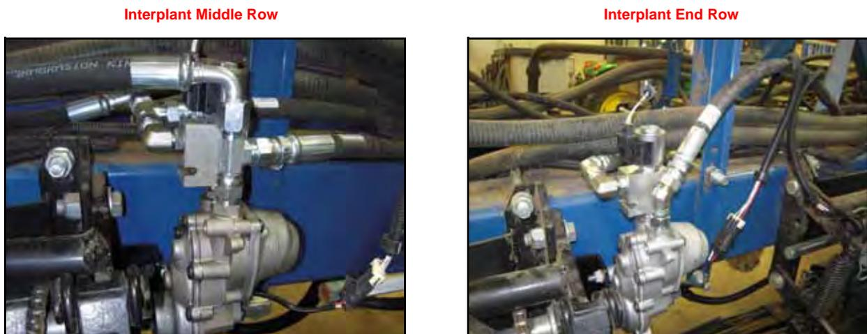
1. Install the supplied hydraulic hoses on each end of the installed tee fittings in Port 2 of the PWM valves, continuing from one row section to the next, until all pressure hoses are installed.
