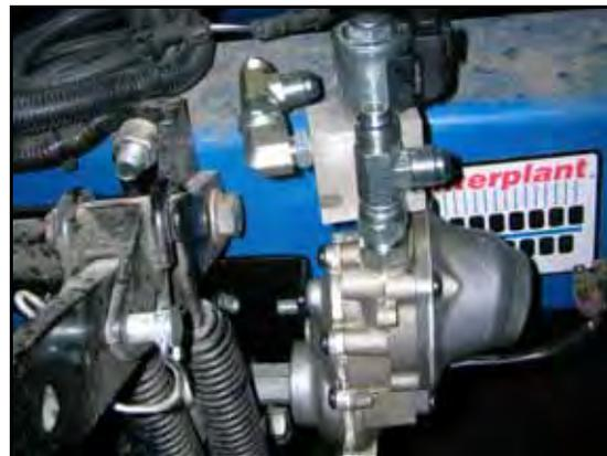
2. Mount the hydraulic motor (P/N 416-8001-001) to the motor mounting bracket using 3/8" x 2-1/2" L bolts (P/N 311-0054-111) and loosely secure with 3/8" zinc flanged lock nuts.
