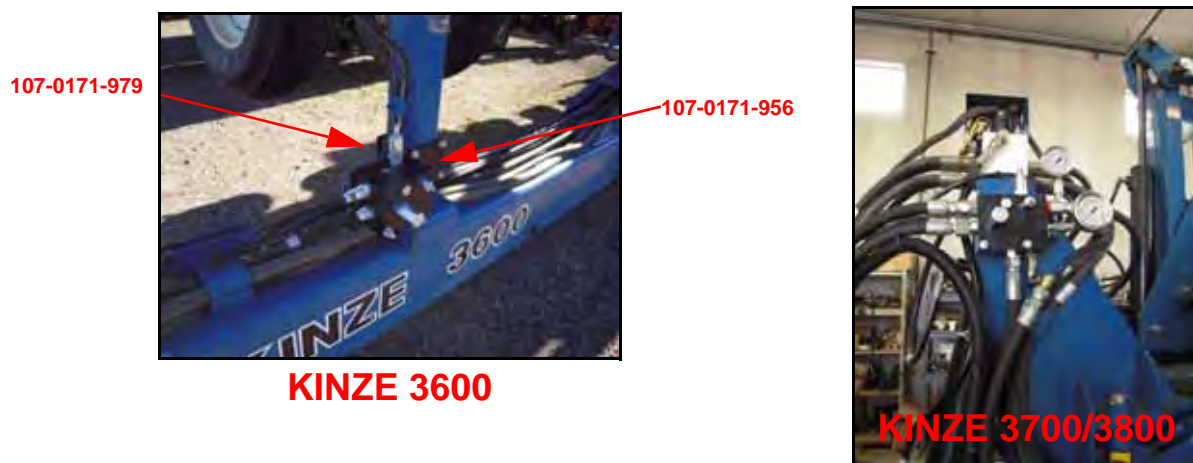
FIGURE 15. Open Center Pressure Reducing Valve Installed on Kinze 3600
