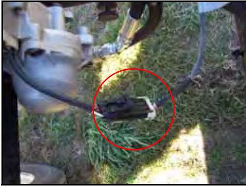
FIGURE 2. Harness Cable Connections on the Row Units
