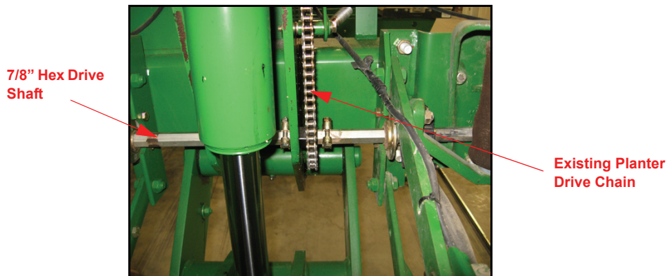
FIGURE 2. Machine's Existing Hex Shaft
