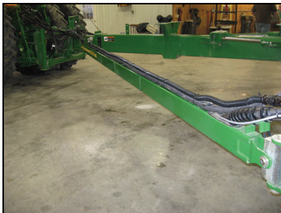
FIGURE 5. Extension Cable Routed to the Tractor Hitch
