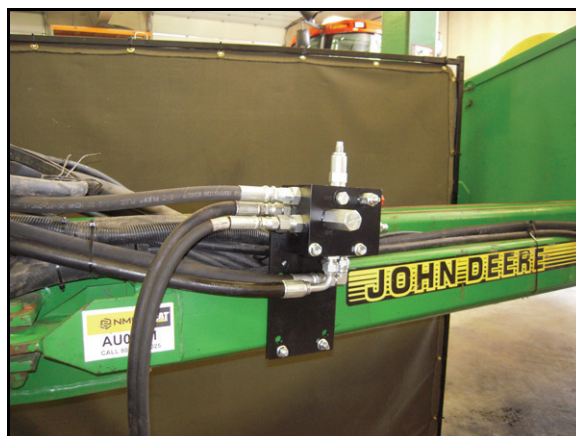
FIGURE 17. Pressure-Reducing Valve Pressure and Tank Hoses Installed
