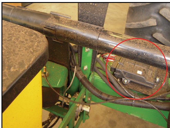
FIGURE 7. OmniRow Node Installed
