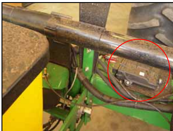
FIGURE 7. OmniRow Node Installed
