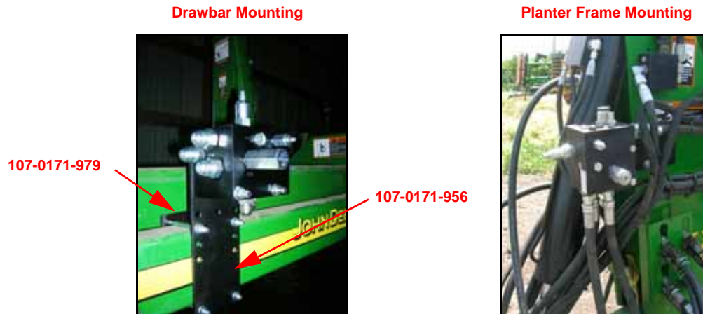
FIGURE 24. OmniRow Valve Installed
