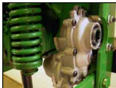
Motor Installed with Factory Heavy-Duty Down Force Springs
