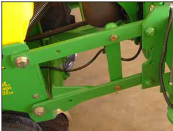
Parallel Linkage Bars on Outside of Row Unit Mounting Bracket (No Spacer Required)
