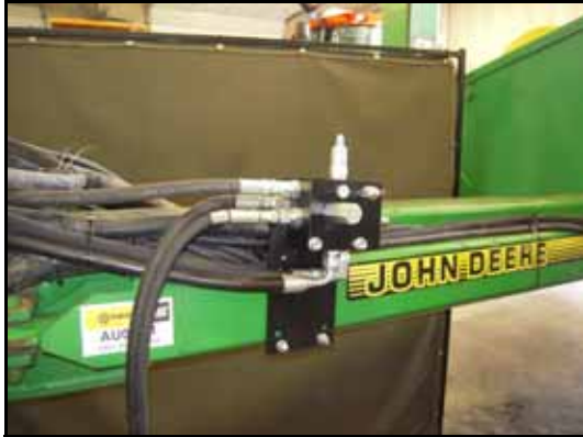
FIGURE 29. OmniRow Valve Pressure and Tank Hoses Installed
