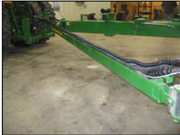
FIGURE 5. Extension Cable Routed to the Tractor Hitch
