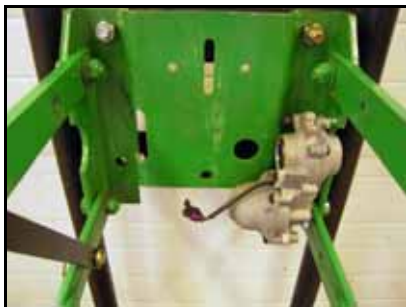
Standard Motor Installation Configuration
