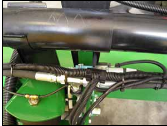
FIGURE 2. Harness Cable Routed to the Planter Row Units
