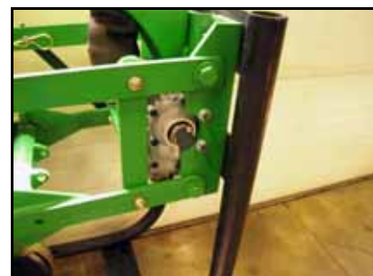
Motor Installed with Factory Airbag Down Pressure
