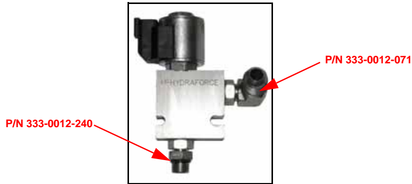
FIGURE 13. Fittings and PWM Valves Installed - End Row Units
