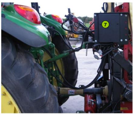
The hydraulic hoses of the Side-Shift cylinder can be mounted directly to the A and B port of the manifold (see previous page) (8).
