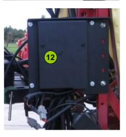
Mount the cover with  $4 \times M8$  bolts and nuts to the hydraulic mounting plate (12).
