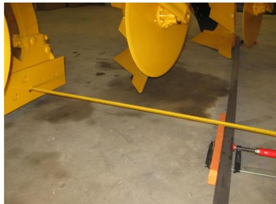
Convert the measured width to the total ploughing width. This should be done by dividing the measured width by the number of measured elements. The result should be multiplied with the total number of elements.
