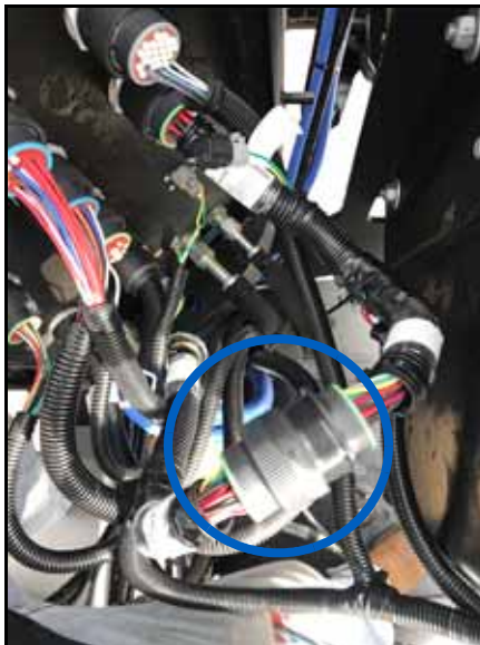
FIGURE 24. RS1 Connected to Machine's Mating Connector
