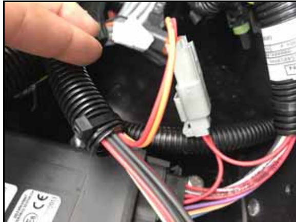
FIGURE 19. 2-Pin Connector on the HDU Valve Cable
