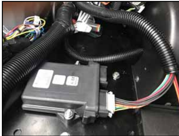
FIGURE 15. 12-Pin Connected to HDUI
