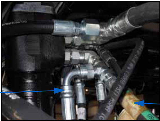
FIGURE 11. Pressure Hose Installed on Steering Orbital
