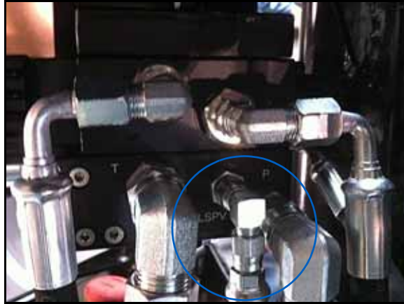
FIGURE 15. LSPV Connection on Steering Valve
