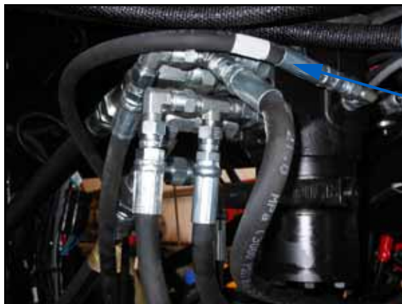
FIGURE 16. Load Sense Hose Installed on Steering Orbital
