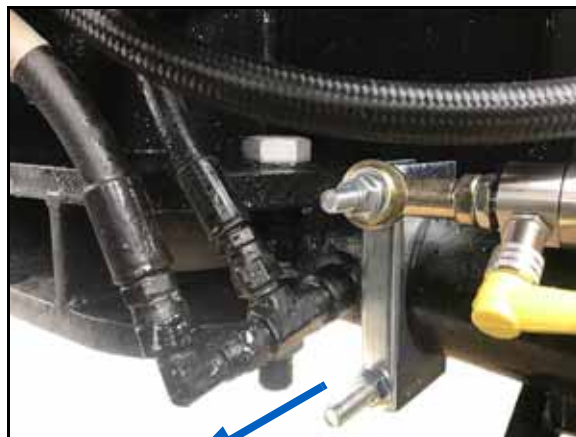
FIGURE 2. U-Bolt Pointing to Front of Machine
