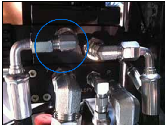
FIGURE 7. Left Steering Hose Installed on Steering Valve
