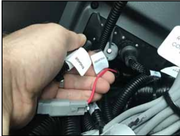
FIGURE 17. 2-Pin Engage to SMARTTRAX Cable
