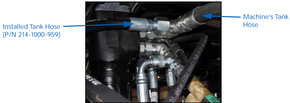
FIGURE 13. Tank Hose Installed on Steering Orbital
