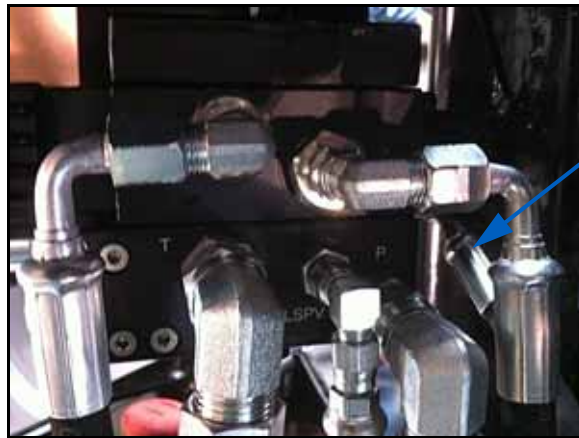
FIGURE 17. LS STEER Connection on Steering Valve
