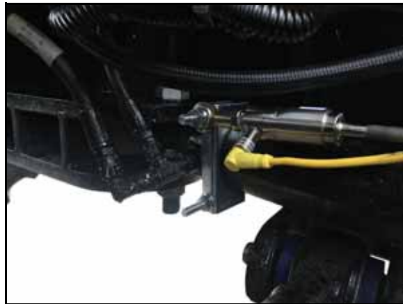
FIGURE 22. WAS Cable Connected to WAS
