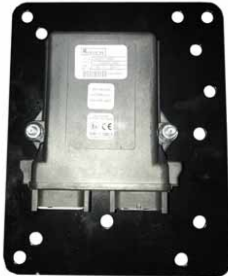
FIGURE 6. HDU Installed on Mounting Plate
