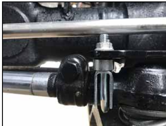
FIGURE 4. U-Bolt on Left Steering Cylinder
