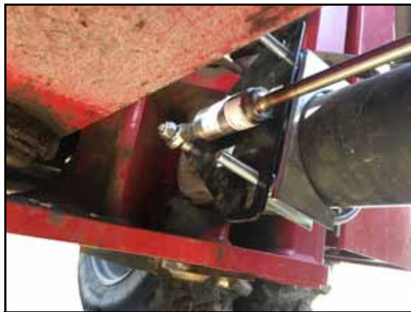
FIGURE 5. Base-End of Sensor Installed
