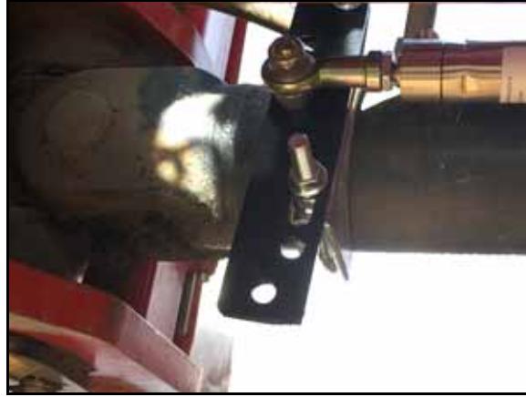
FIGURE 10. Base-End of WAS Installed
