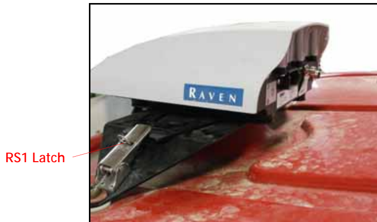
FIGURE 3. Installed RS1 Unit
