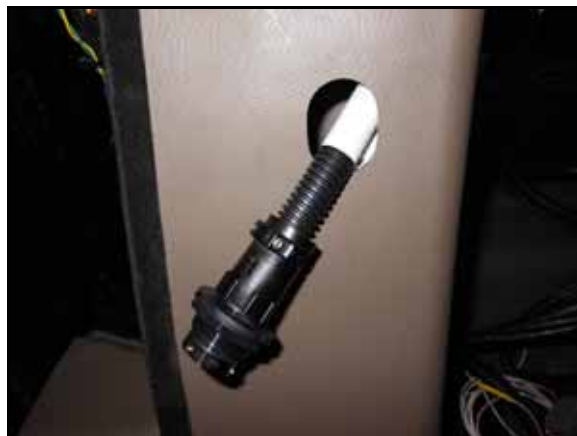
FIGURE 24. ISO Bus Display Adapter Harness Routed Through Post Cover
