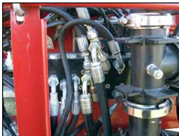
FIGURE 4. Left and Right Down Hoses Installed
