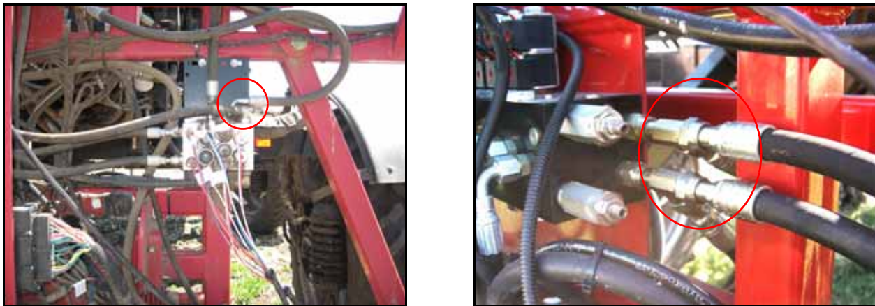
FIGURE 2. Pressure and Tank Hoses Installed
