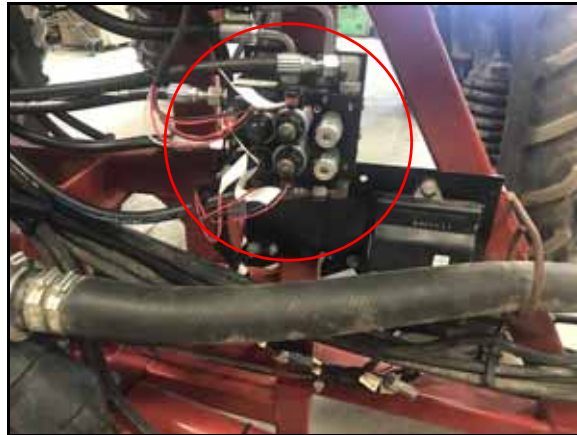
FIGURE 1. AutoBoom Valve Mounted to the Center Rack
