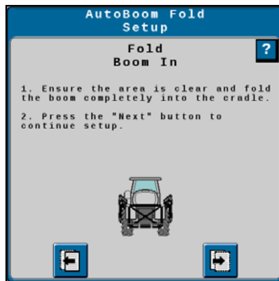
FIGURE 26. AutoBoom Fold Setup- Fold Boom In
