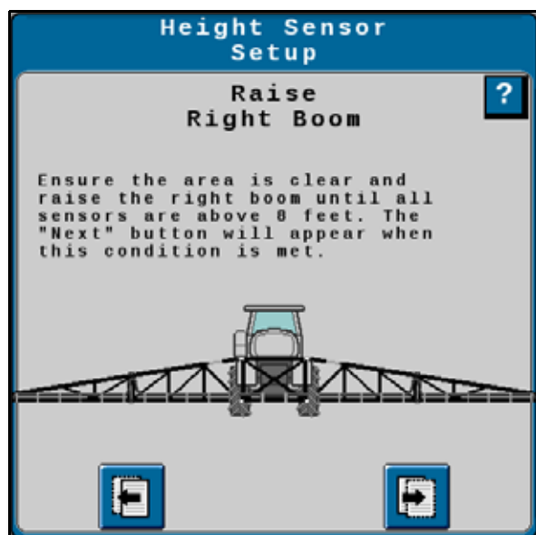
FIGURE 24. Height Sensor Setup - Raise Right Boom
