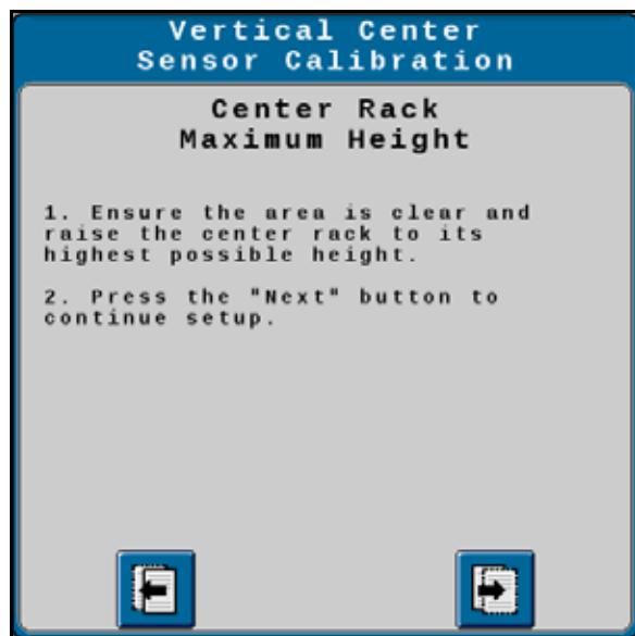
FIGURE 6. Vertical Center Sensor Calibration - Maximum Height
