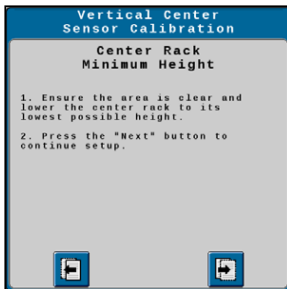
FIGURE 9. Vertical Center Sensor Calibration - Minimum Height
