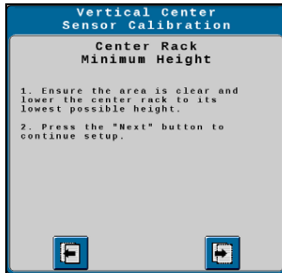
FIGURE 30. Vertical Center Sensor Calibration - Minimum Height
