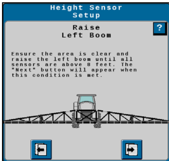
FIGURE 23. Height Sensor Setup - Raise Left Boom
