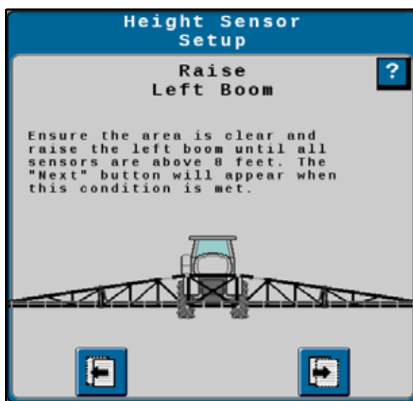
FIGURE 15. Height Sensor Setup - Raise Left Boom
