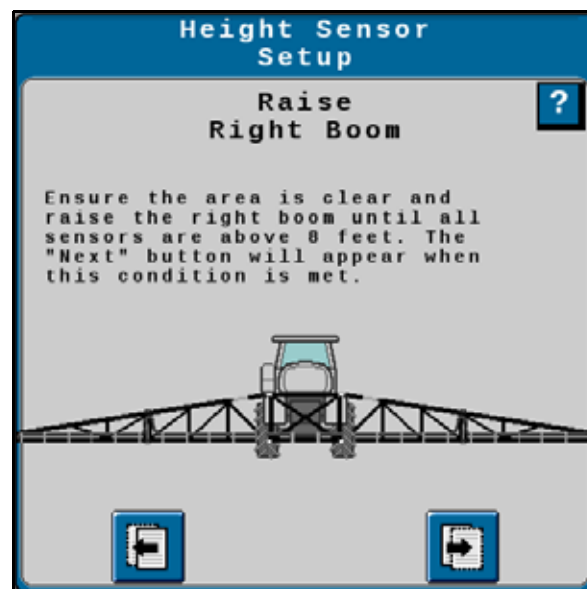
FIGURE 18. Height Sensor Setup - Raise Right Boom
