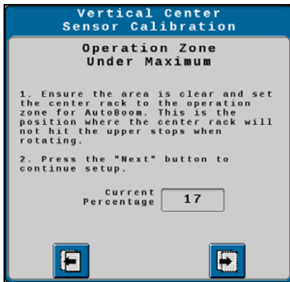
FIGURE 28. Vertical Center Sensor Calibration - Operation Zone
