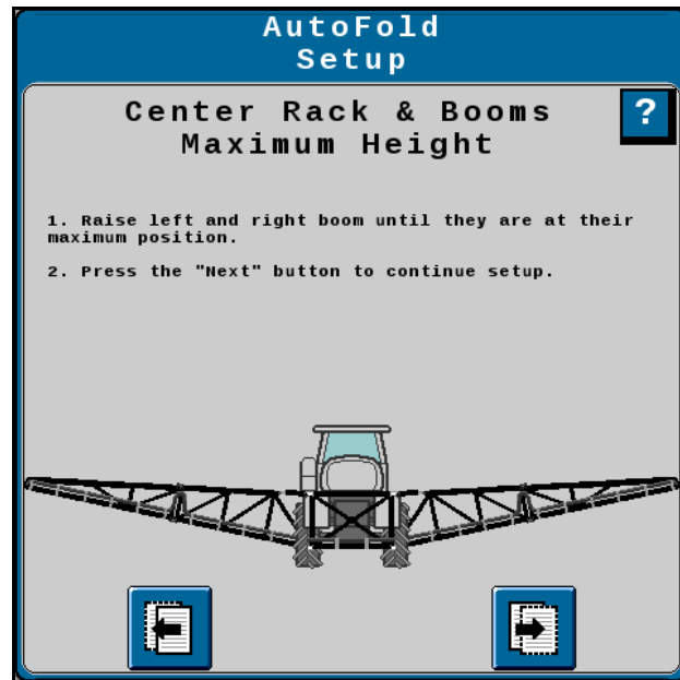
FIGURE 35. Raise Center Rack and Booms
