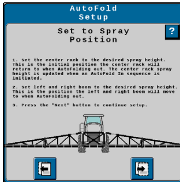
FIGURE 37. Set Booms and Center Rack to Spray Position
