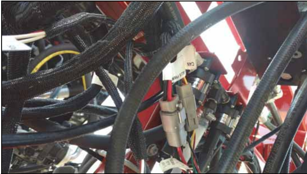
FIGURE 11. CAN and PWR Connections
