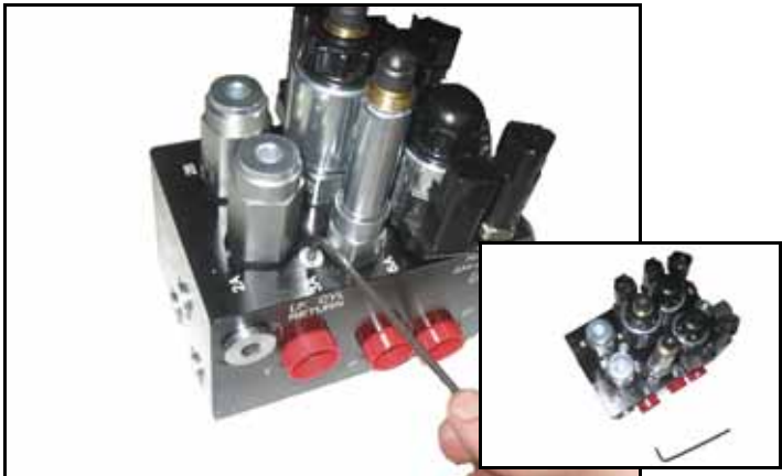
FIGURE 3. Port Plugs Removed from the AutoBoom Valve
