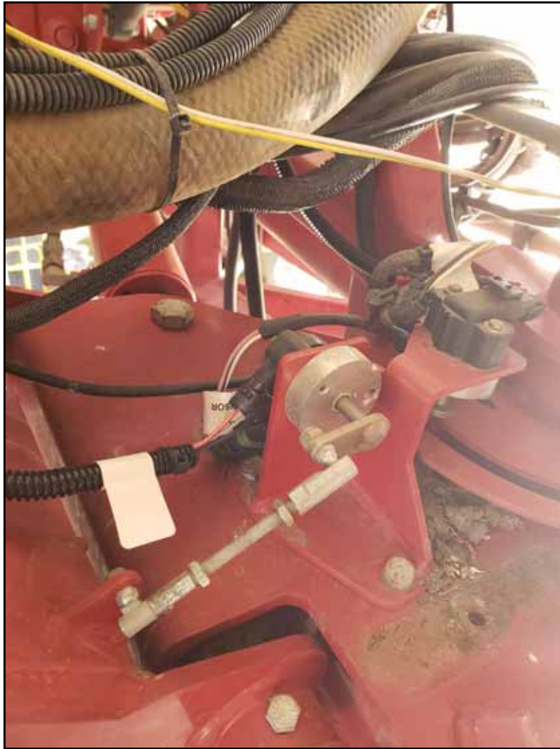
FIGURE 20. Tilt and Fold Harness Connections
