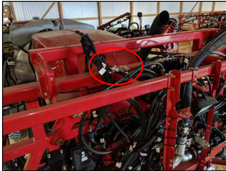
FIGURE 6. CAN and PWR Connections
