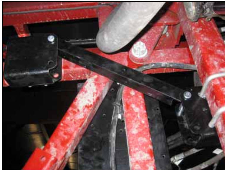
FIGURE 18. Damper Brackets Loosely Installed with Damper Spacing Template
