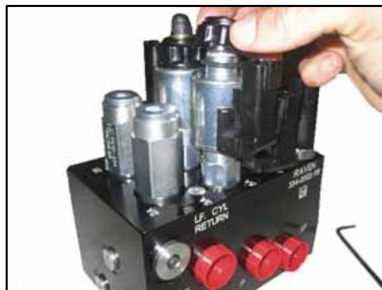
FIGURE 6. Coil Reinstalled on the AutoBoom Valve
