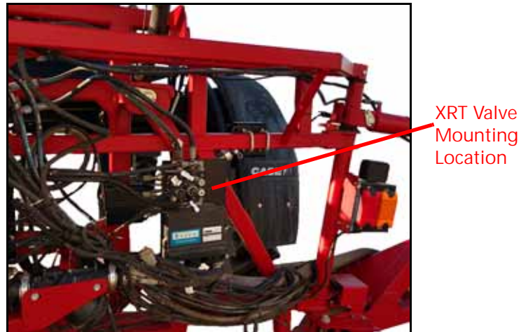
FIGURE 7. XRT Valve Mounting Location
