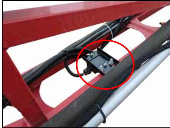
FIGURE 3. Inner Boom Sensor Installed (120' Steel Boom Shown)
