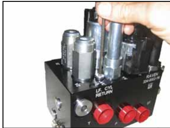
FIGURE 5. Port Plug Reinstalled on the AutoBoom Valve
