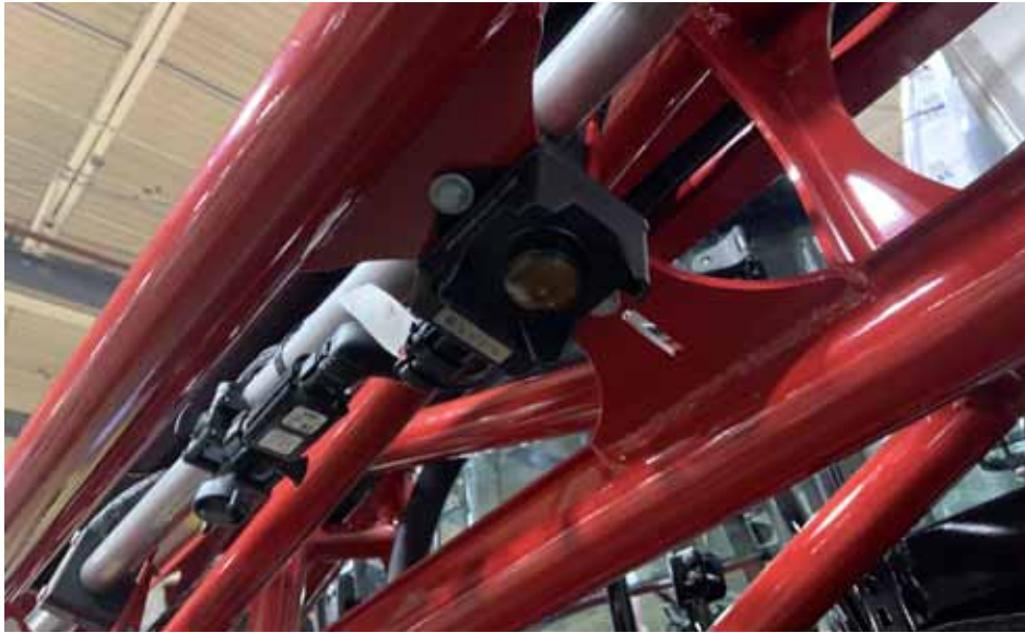
FIGURE 8. Inner Boom Sensor Installed
