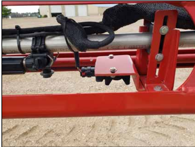
FIGURE 6. Example of the Radar Sensor Installed at the Right Boom Tip
