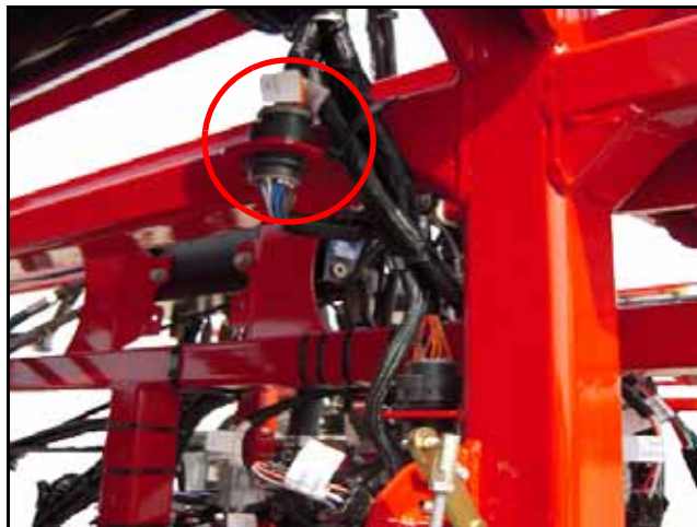
FIGURE 7. AutoBoom Harness Cable Installed
