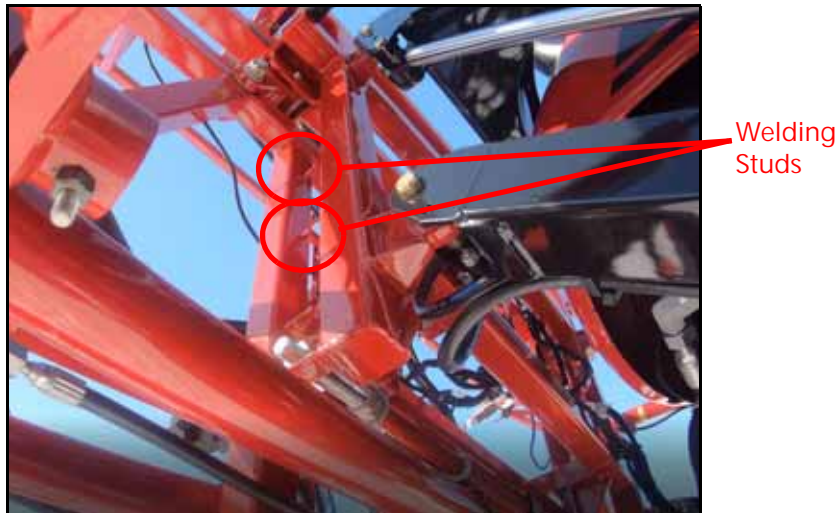
FIGURE 16. Damper Installation Location
