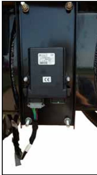
FIGURE 5. AutoBoom Cable Connected to Node
