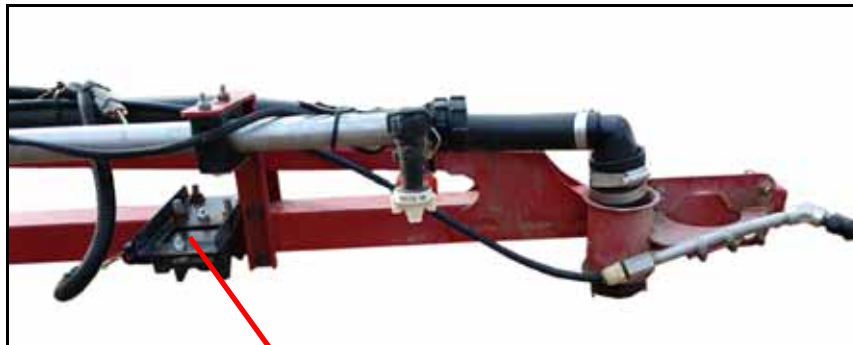
FIGURE 2. Boom Sensor Installed
