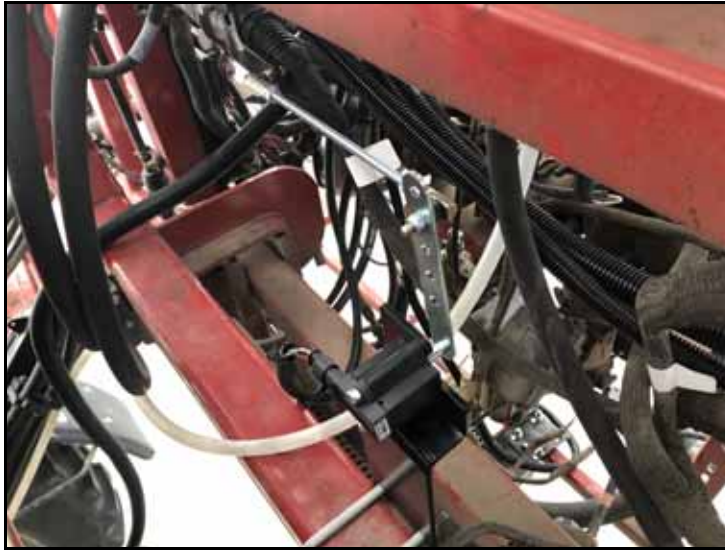
FIGURE 15. Rotary Sensor Installation Location on Center Rack
