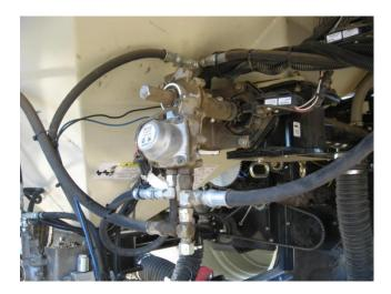
• Mount hydraulic motor and pwm valve to bracket.
