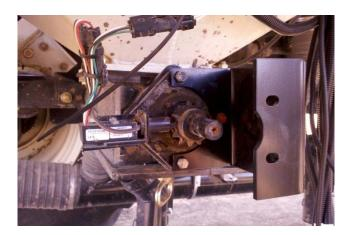
• For middle bins mount bracket so holes are aligned vertically, but to the left side of the meter shaft such that the motor will have its fittings pointing downward once installed.
