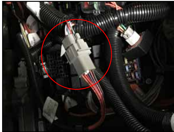
FIGURE 8. HDU Harness Cable Connection
