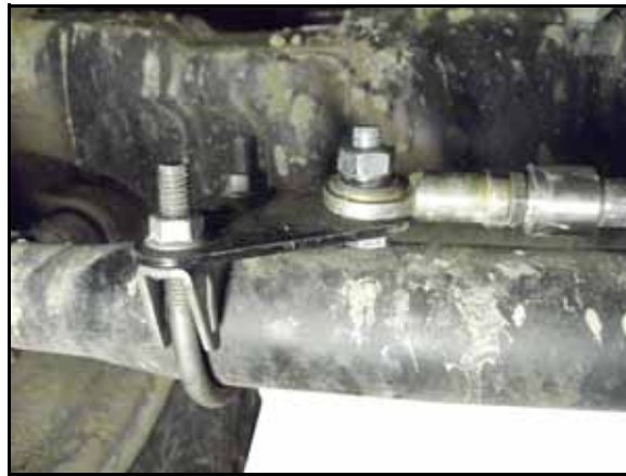
FIGURE 3. Rod End of the WAS Secured to the WAS Bracket
