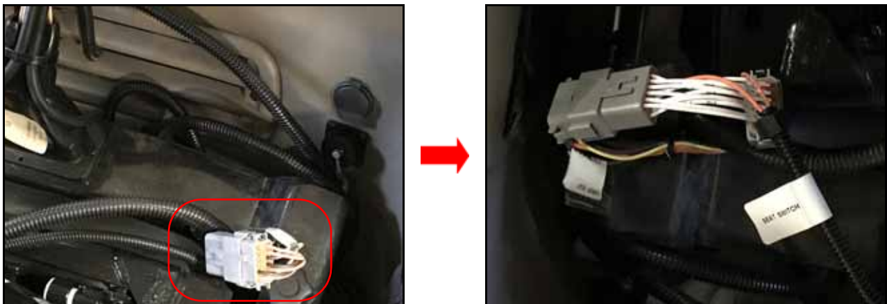
FIGURE 9. Seat Switch Harness Connections
