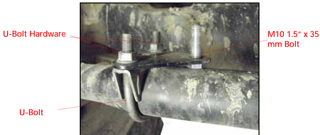
FIGURE 2. Rod End of the WAS Secured to the WAS Bracket
