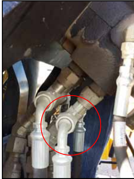
FIGURE 5. Right Steering Hose Installed on Steering Orbital
