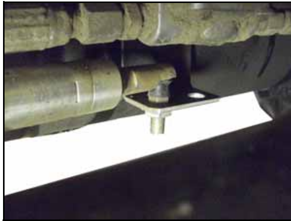
FIGURE 5. Base End Installed in the WAS Bracket
