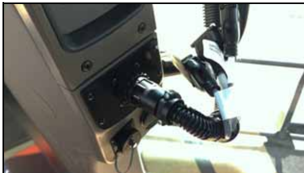
FIGURE 19. 16-Pin on Harness Cable Connection
