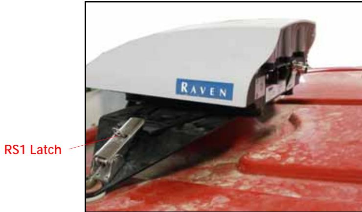
FIGURE 3. Installed RS1 Unit
