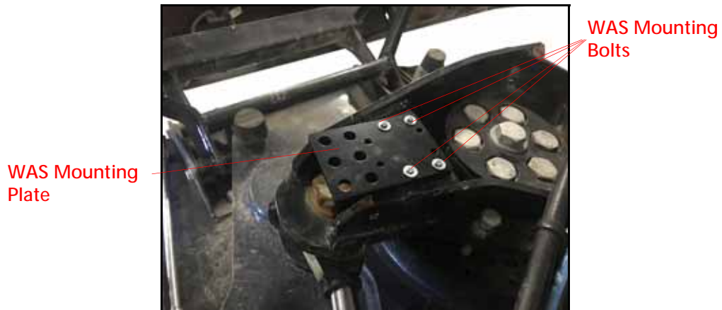
FIGURE 3. WAS Mounting Plate Installed on the Pivot Point
