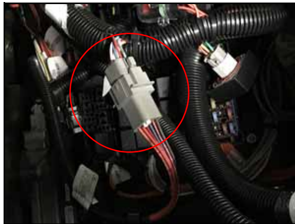
FIGURE 8. HDU Harness Cable Connection
