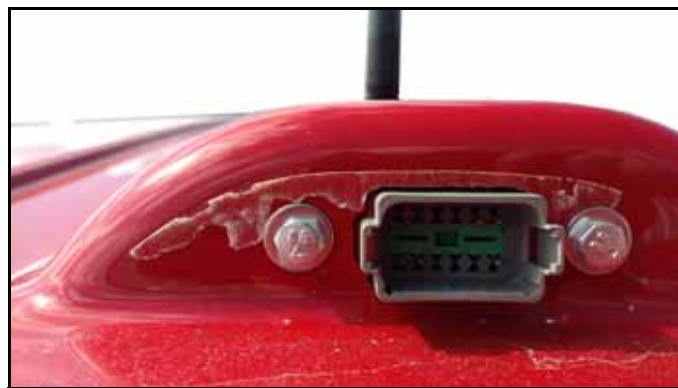
FIGURE 4. Connector Cutout Installation
