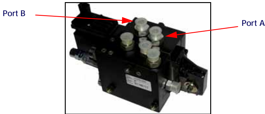
FIGURE 1. Fittings Installed in the Valve
