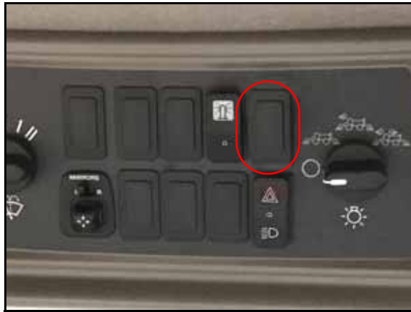
FIGURE 10. Master Switch Installation Location
