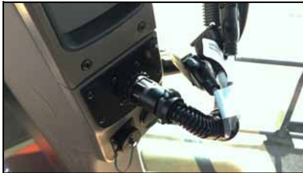
FIGURE 19. 16-Pin on Harness Cable Connection
