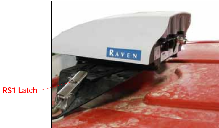
FIGURE 3. Installed RS1 Unit
