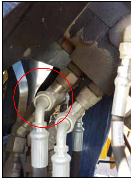
FIGURE 4. Left Steering Hose Installed on Steering Orbital
