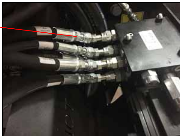
FIGURE 8. Pressure Hose Installed on Valve
