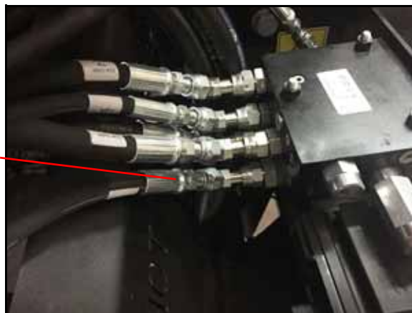
FIGURE 6. Right Steering Hose Installed on Valve
