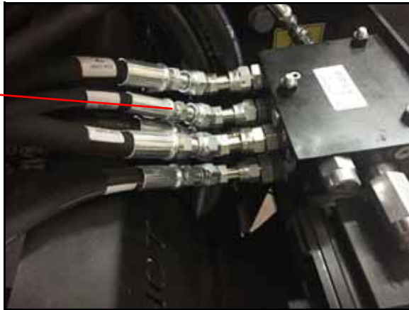
FIGURE 12. Load Sense Hose Installed on Steering Orbital
