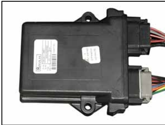
FIGURE 6. HDU Harness Cable Installed on HDU
