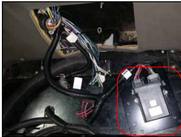
FIGURE 10. HDU Installed on HDU Mounting Bracket
