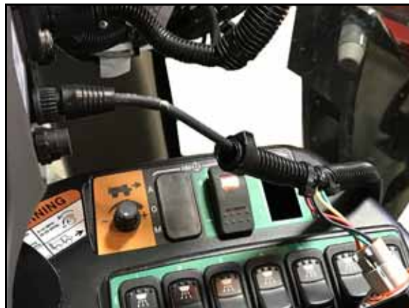
FIGURE 8. RS1 HDU Harness Connected to Viper 4 Field Computer
