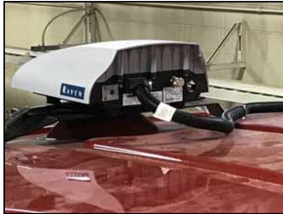
FIGURE 3. RS1 Unit Installed on Cab Roof
