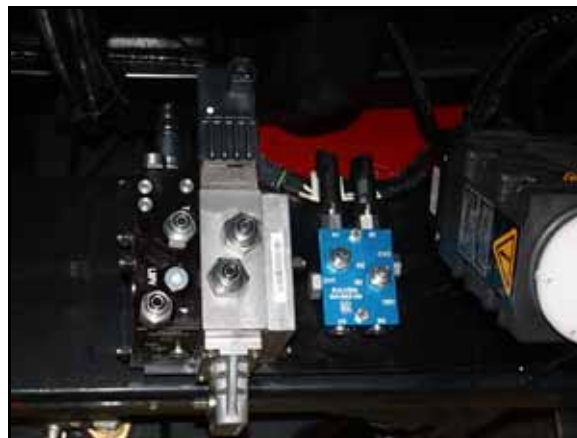
FIGURE 5. Steering Valve Mounted on the Machine
