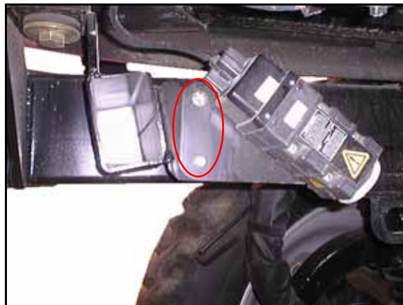
FIGURE 3. Mounting Bracket Installed
