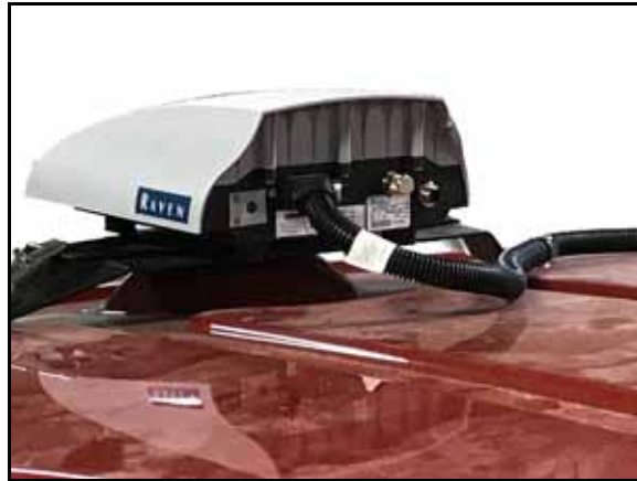
FIGURE 3. RS1 Unit Installed on Cab Roof
