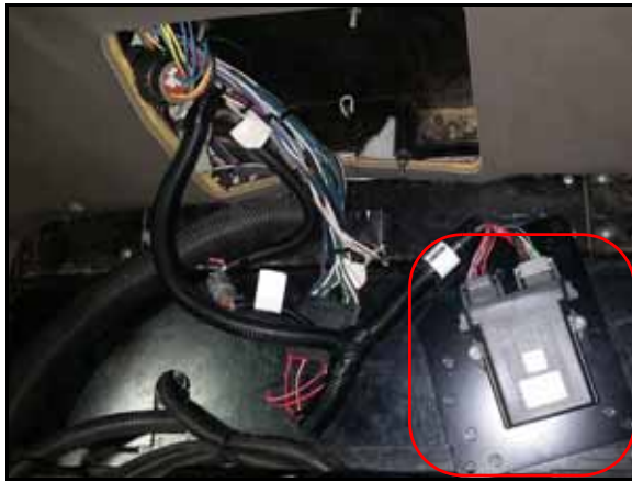
FIGURE 17. HDU Installed on HDU Mounting Bracket
