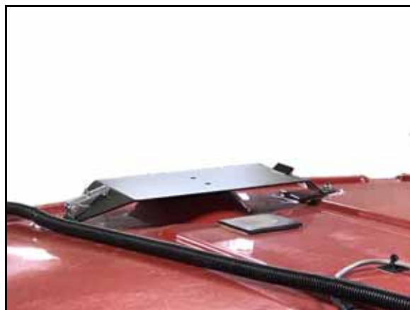
FIGURE 2. Machine's Existing Receiver Mounting Bracket
