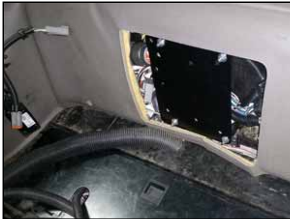
FIGURE 18. HDU Mounting Bracket Installed
