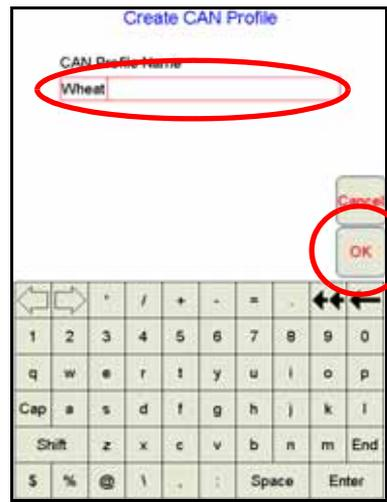
4. To save a CAN Profile, touch the **Create CAN Profile** button. Using the on-screen keyboard, enter a **profile name** and touch **OK**.
