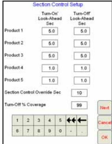
2. Select the **Look-Ahead**, **Override Sec**, or **Turn-Off % Coverage** fields to modify and use the on-screen keypad to enter the desired value.
