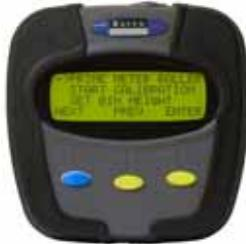
3. Press the **Enter** key to select the 'Prime Meter Roller' option and then press the **Start** key to begin priming the metering rollers.
