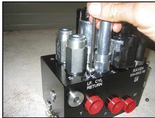
FIGURE 5. Port Plug Reinstalled on the AutoBoom Valve
