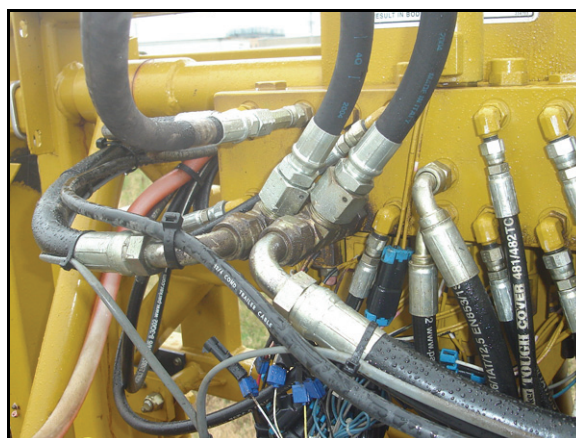
FIGURE 10. Left and Right Cylinder Hoses Installed
