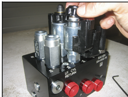
FIGURE 6. Coil Reinstalled on the AutoBoom Valve
