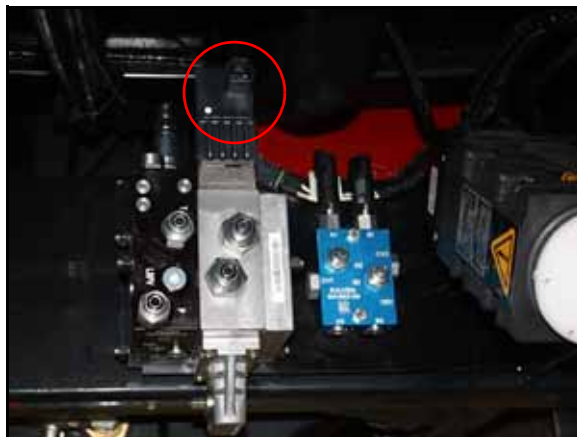
FIGURE 18. VALVE Harness Cable Installation Location
