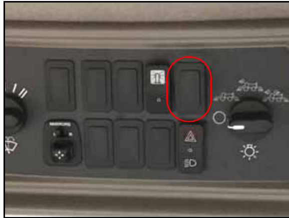
FIGURE 11. Master Switch Installation Location
