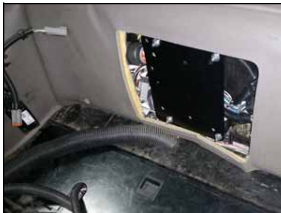
FIGURE 14. HDU Mounting Bracket Installed
