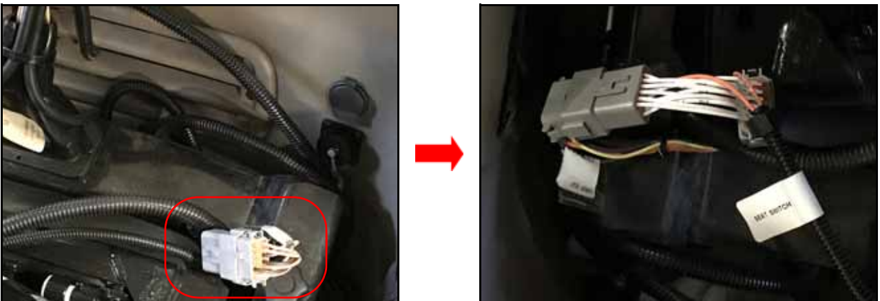
FIGURE 10. Seat Switch Harness Connections
