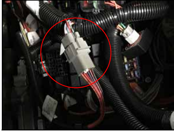
FIGURE 9. HDU Harness Cable Connection
