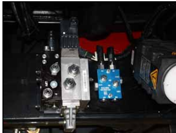
FIGURE 5. Steering Valve Mounted on the Machine
