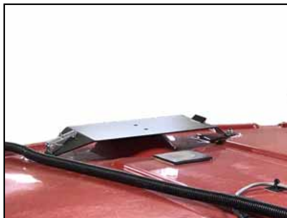
FIGURE 2. Machine's Existing Receiver Mounting Bracket
