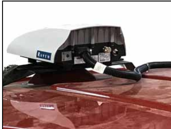
FIGURE 3. RS1 Unit Installed on Cab Roof
