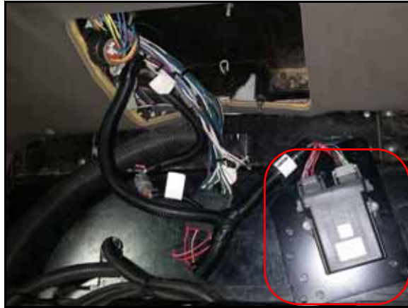
FIGURE 13. HDU Installed on HDU Mounting Bracket
