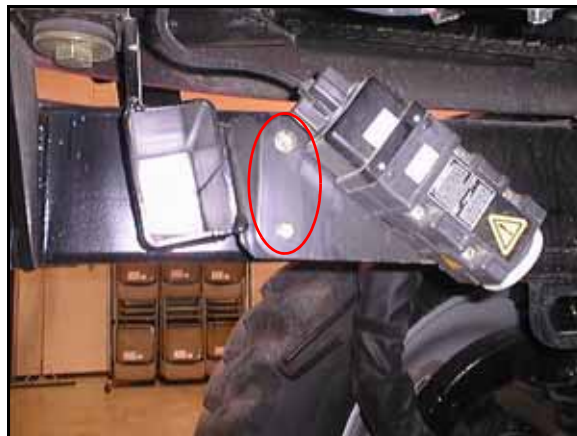
FIGURE 3. Mounting Bracket Installed
