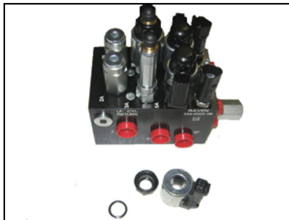
FIGURE 2. Coil Removed from the AutoBoom Valve
