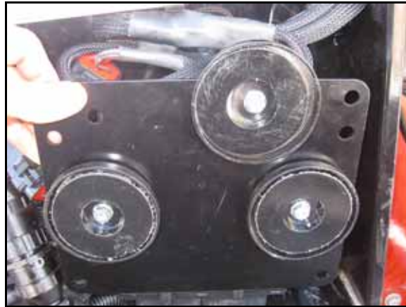
FIGURE 2. Magnets Installed on Node Mounting Bracket
