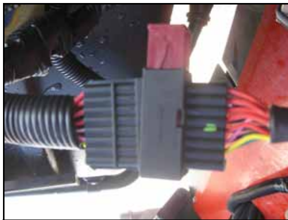
FIGURE 8. Machine's ECU Connectors Connected to Raven ISO Tee Adapter Cable
