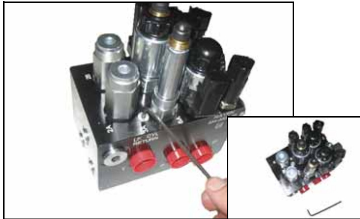
FIGURE 3. Port Plugs Removed from the AutoBoom Valve
