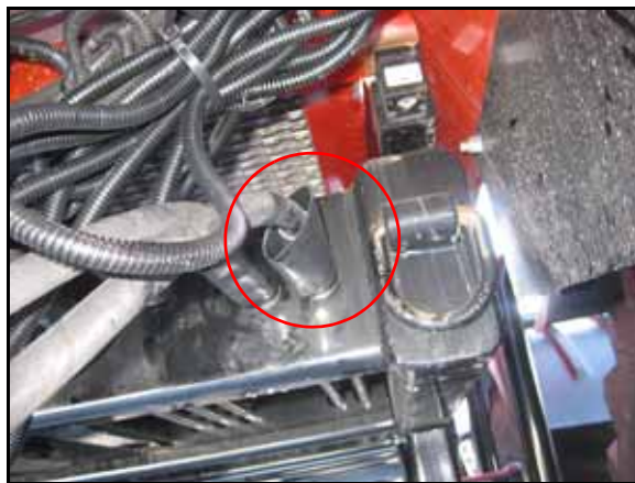
FIGURE 16. Pressure Hose Installed on Machine's Open Port
