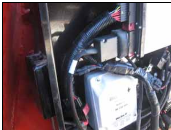
FIGURE 9. Raven ISO Tee Adapter Cable Installed on Machine's ECU
