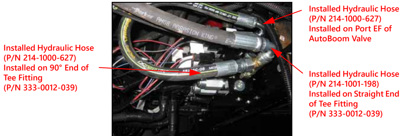
FIGURE 19. Tank Hose Installed on AutoBoom Valve
