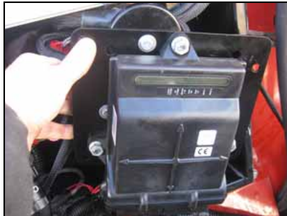
FIGURE 3. Node Installed on Node Mounting Bracket
