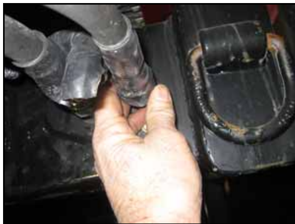
FIGURE 12. Heat Shrink Tubing Removed from Hose
