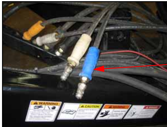
FIGURE 17. Machine's Pressure SCV Connection
