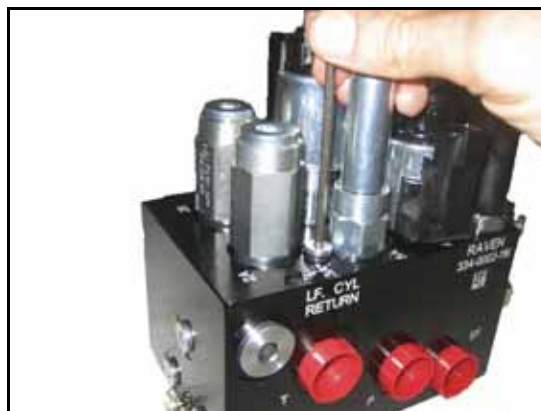
FIGURE 5. Port Plug Reinstalled on the AutoBoom Valve
