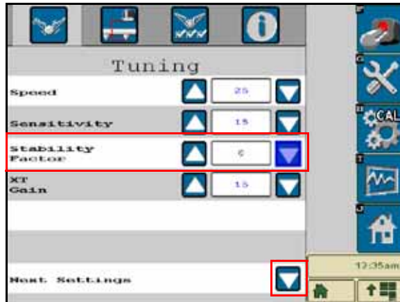
FIGURE 3. Stability Factor Setting Adjustment
