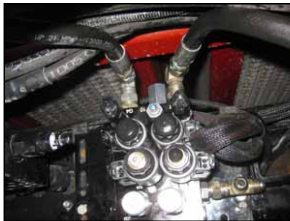
FIGURE 10. Valve Installed on Machine's Cross-member
