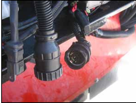
FIGURE 10. Raven ISO Tee Adapter Cable and AutoBoom Harness Connections
