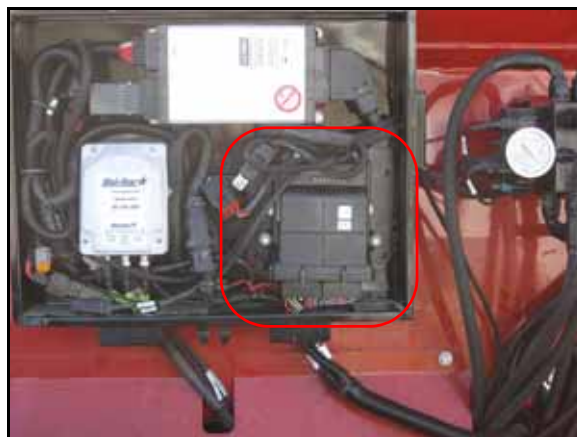
FIGURE 4. Node Mounted in Electrical Box
