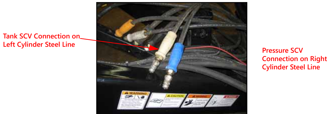
FIGURE 20. Machine's Tank SCV Connection
