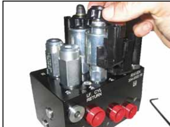
FIGURE 6. Coil Reinstalled on the AutoBoom Valve
