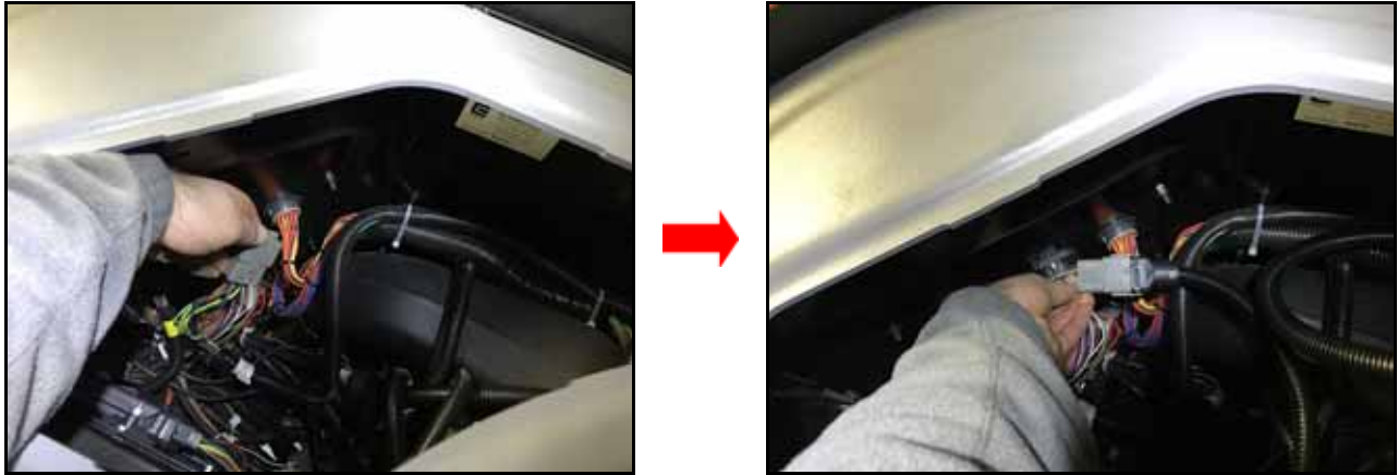
FIGURE 9. GPS POWER/CAN Connector
