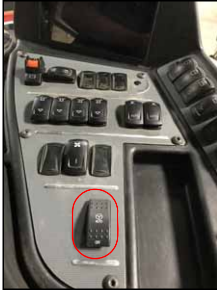
FIGURE 17. Steering Lockout Switch Installed
