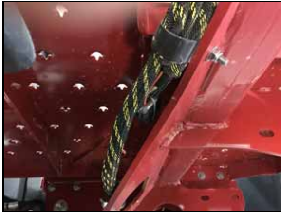
FIGURE 21. Steering Lockout Cable Routing
