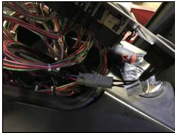
FIGURE 16. STEERING LOCKOUT SWITCH Connector
