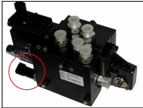
FIGURE 1. Pressure Transducer to be Removed
