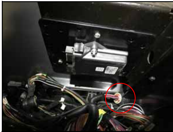
FIGURE 10. HDU Harness Bulkhead Connector Connected to Machine's Bulkhead
