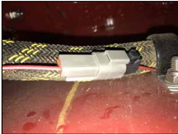
FIGURE 22. Steering Lockout Cable Connection
