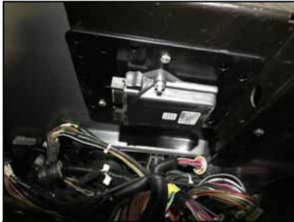
3. Install the HDU mounting bracket (P/N 107-0172-543) on the machine's existing plate using three M6 1.0 x 20 mm class 5.8-8.8 flanged bolts (P/N 311-0070-051).
