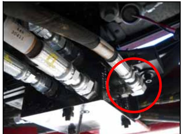
3. Install the straight end of the supplied hydraulic hose (P/N 214-1000-949) on the existing 90° elbow fitting in the load sense port of the machine's steering orbital.
