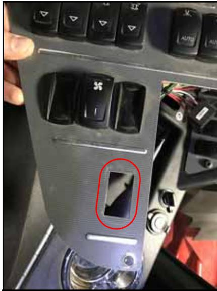
8. Identify an open port on the machine's side console cover.
