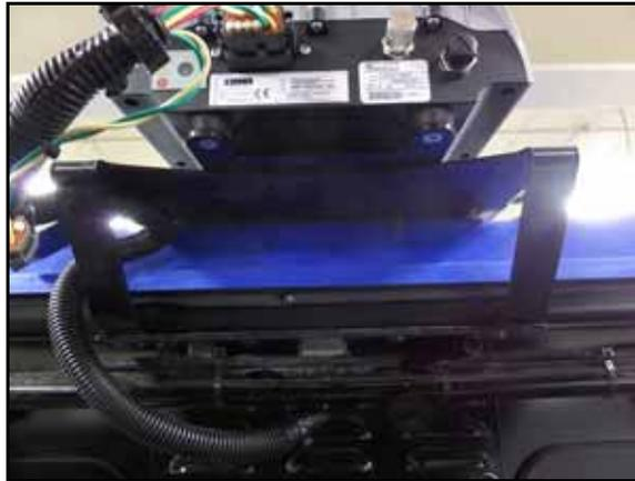
2. Connect the other end of the RS1 harness to the machine's bulkhead connector.
