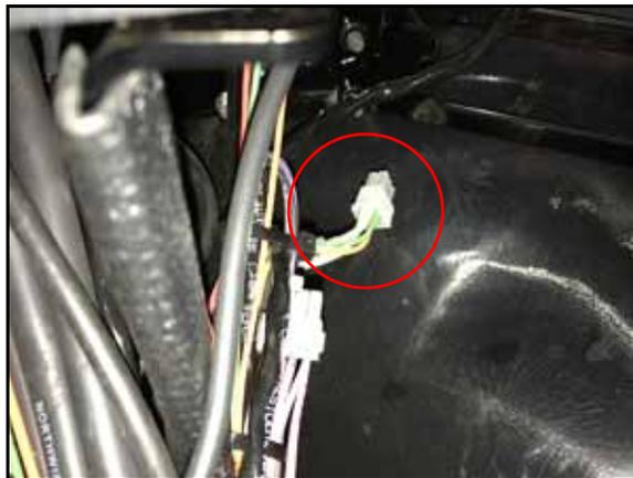
7. Connect the J1939 CAN connector of the HDU harness to the machine's mating AR193 connector.
