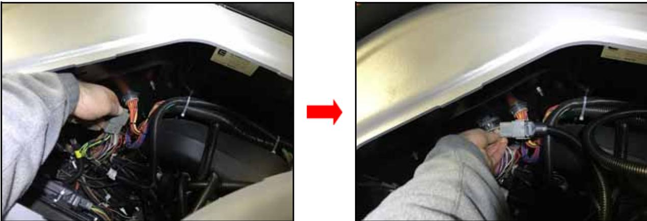
1. Trace the cable from the machine's GPS bulkhead connector down the rear wall of the machine and into the instructional seat compartment.
