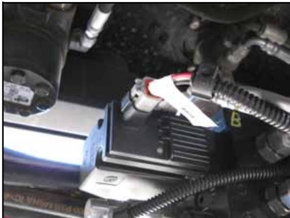
3. Connect the PVES connector to the open PVES port on the end of the steering valve.
