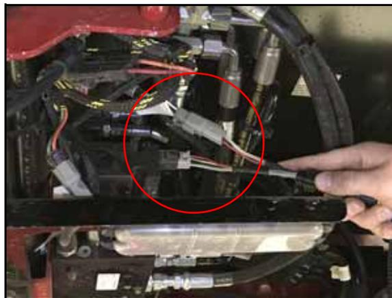
1. Disconnect the PVES connector of the valve harness (P/N 115-4001-140) from the steering valve.
