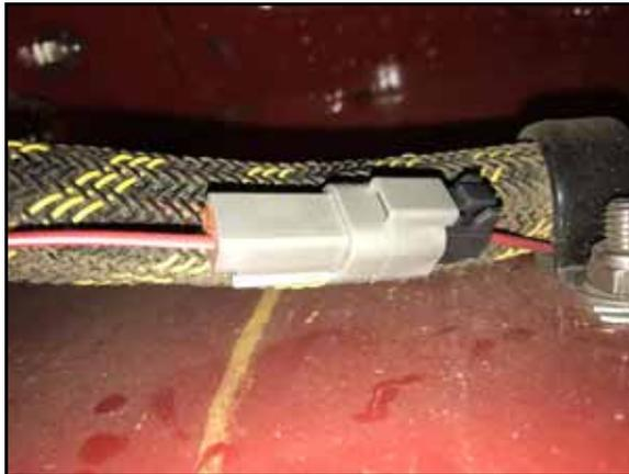
5. Connect the TO MACHINE'S FOUR WHEEL STEER (FW355) CONNECTOR to the machine's FW355 connection.
