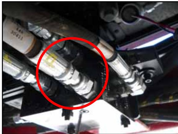
5. Connect the straight end of the installed hydraulic hose to the fitting installed in Port P of the steering valve (P/N 334-0003-094).
