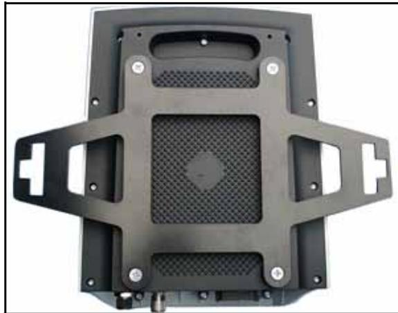
1. Install the RS1 mounting bracket (P/N 107-0172-498) on the bottom of the RS1 unit using four 1/4"-20 x 1/2" flat head machine screws (P/N 311-0003-041).
