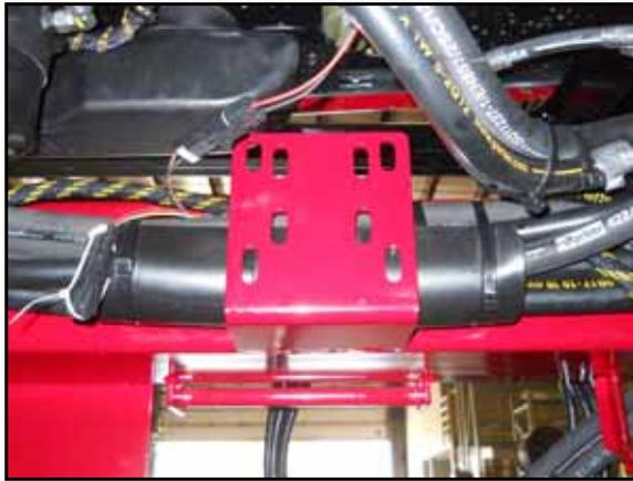
1. Locate the machine's existing mounting plate on the machine's front cross-member, to the right of the steering orbital.
