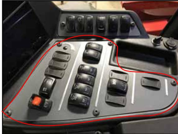
6. Remove the cover from the machine's side console.
