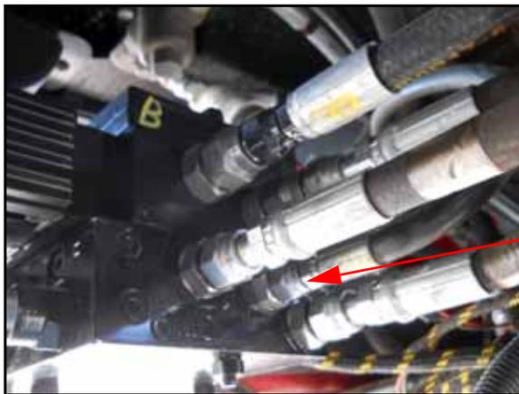
2. Connect the load sense hose to the fitting installed in Port LSPV of the steering valve (P/N 334-0003-094).
