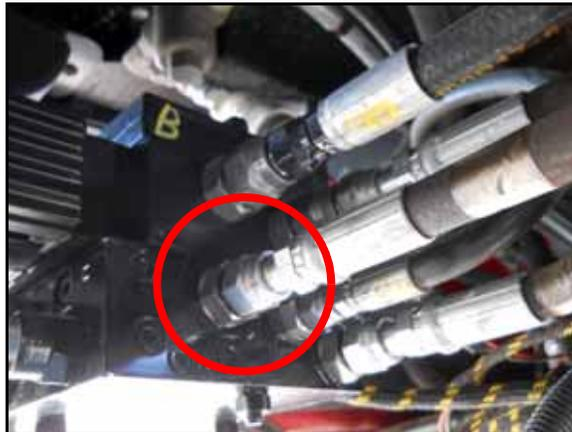
10. Connect the straight end of the installed hydraulic hose to the fitting installed in Port T of the steering valve.
