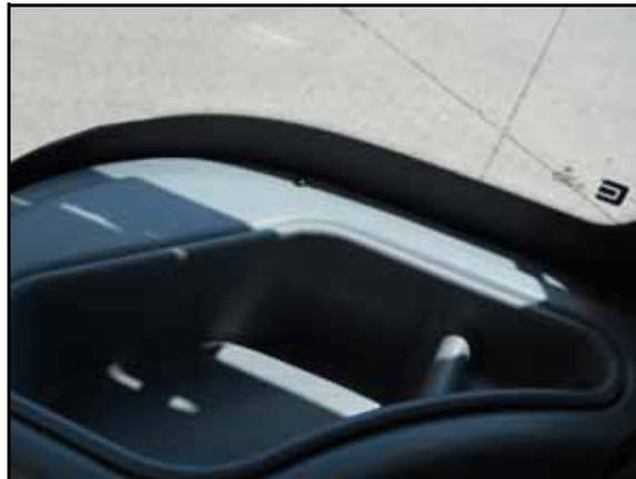
1. Remove the plastic tray located in the right-rear corner of the cab.
