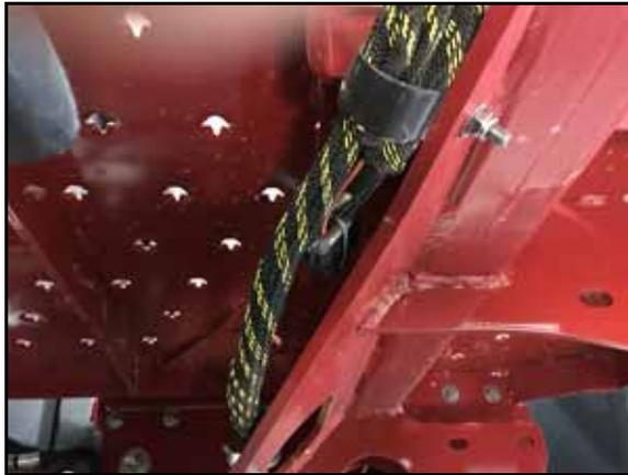
4. Route the remaining connector to the left-rear tire of the machine.
