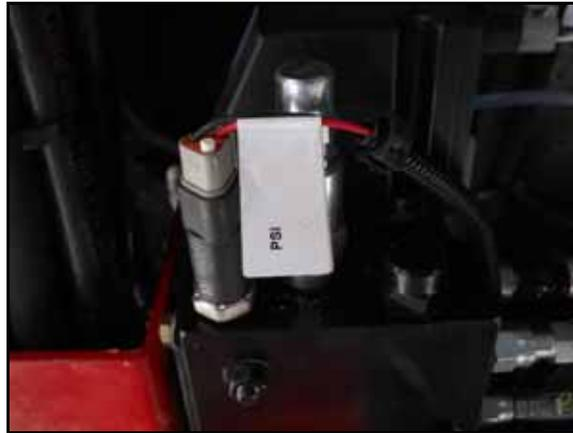
4. Connect the PSI connector to the transducer (P/N 422-0000-086) installed in Port PS of the steering valve.
