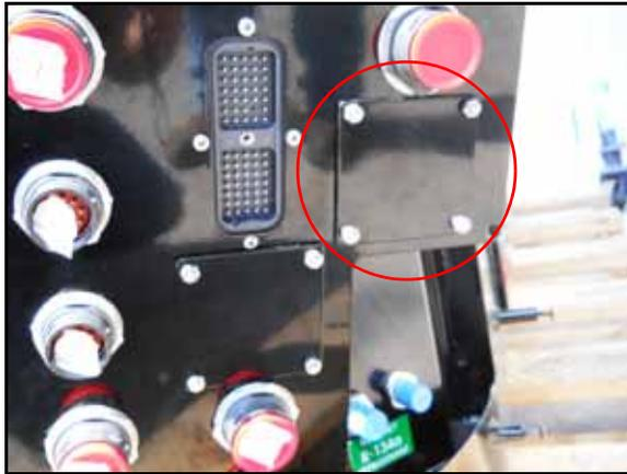
14. Remove the cover plate from the bulkhead as shown in the figure above.
