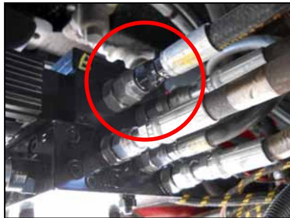
6. Disconnect the machine's right steering hose from the steering orbital.
