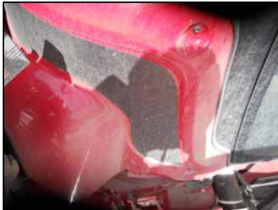
13. Remove the plastic shroud located on the outside of the machine, in the right-rear corner of the cab.
