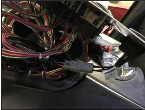
9. Position the master switch (P/N 063-0173-961) over the open port in the side console cover, feeding the switch cable through the opening.
