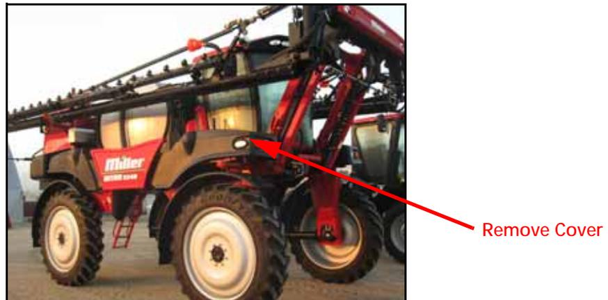
3. Remove the plastic cover from the top of the front right wheel to gain access to the steering cylinder area.
