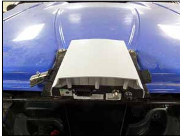
3. Insert the tab of the RS1 latch mounting bracket into the slotted tab of the receiver mounting bracket to interlock the brackets.
