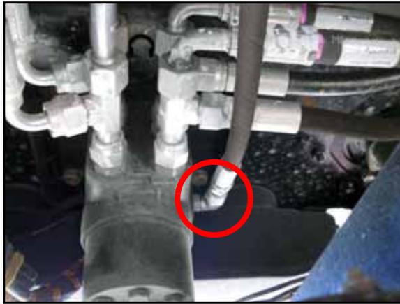
1. Disconnect the machine's load sense hose from the steering orbital.
