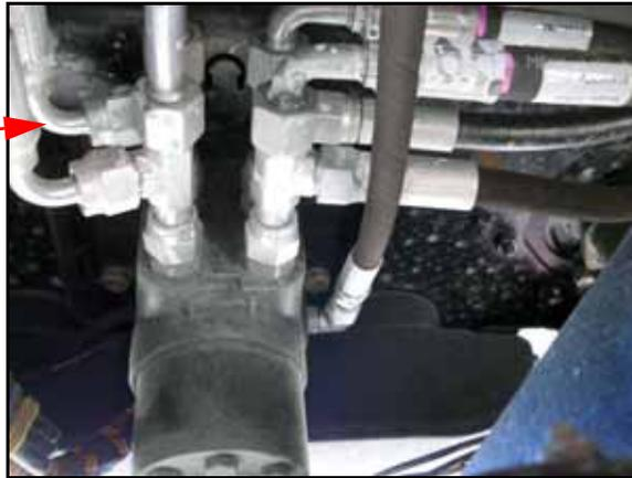
6. Disconnect the machine's tank hose from the steering orbital.
