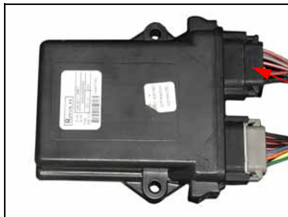
FIGURE 16. RS1 to Bulkhead Cable Installed on HDU
