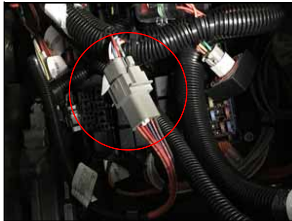
FIGURE 12. HDU Harness Cable Connection
