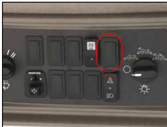
FIGURE 14. Master Switch Installation Location
