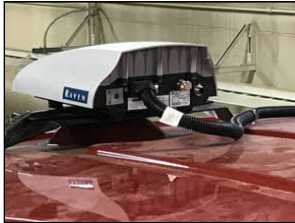
FIGURE 3. RS1 Unit Installed on Cab Roof
