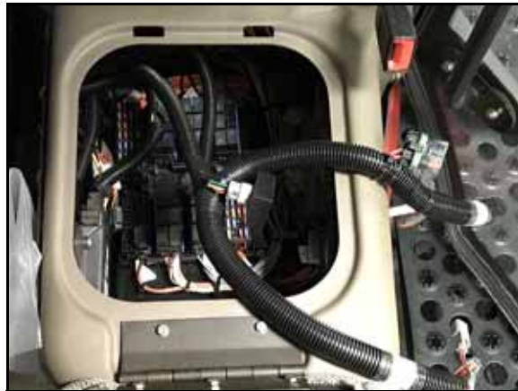
FIGURE 6. RS1 HDU Harness in Instructional Seat Compartment
