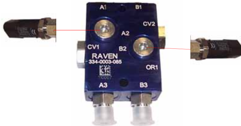
FIGURE 2. Fittings Installed on the Flow Switch
