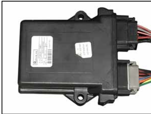
FIGURE 6. HDU Harness Cable Installed on HDU
