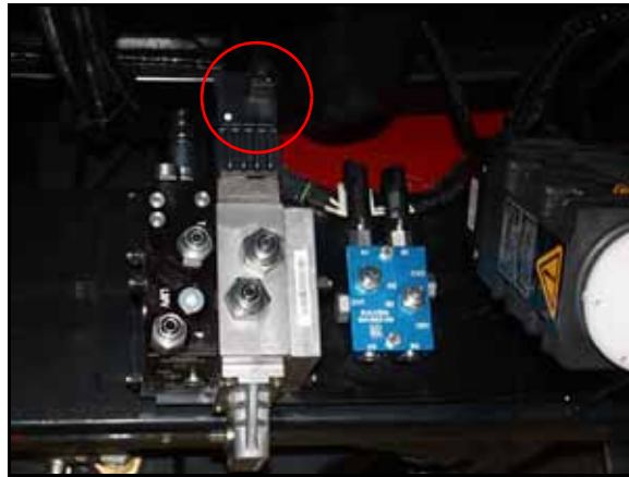
FIGURE 12. VALVE Harness Cable Installation Location
