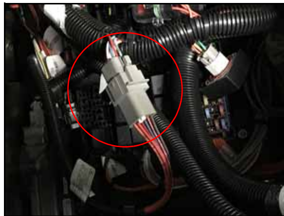
FIGURE 8. HDU Harness Cable Connection
