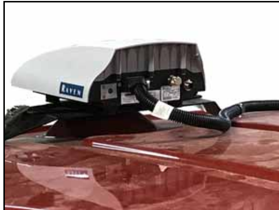
FIGURE 3. RS1 Unit Installed on Cab Roof
