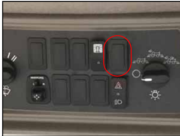
FIGURE 10. Master Switch Installation Location
