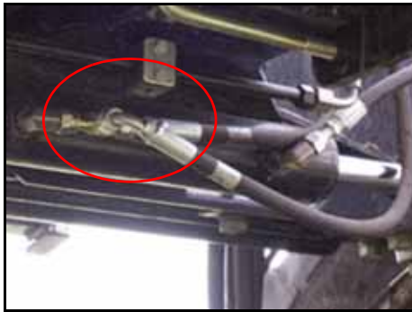
FIGURE 10. Raven Steering Hose Installed
