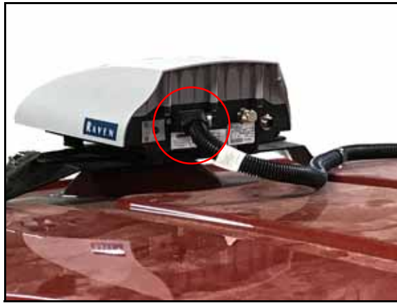
FIGURE 18. RS1 Tee Cable Connection
