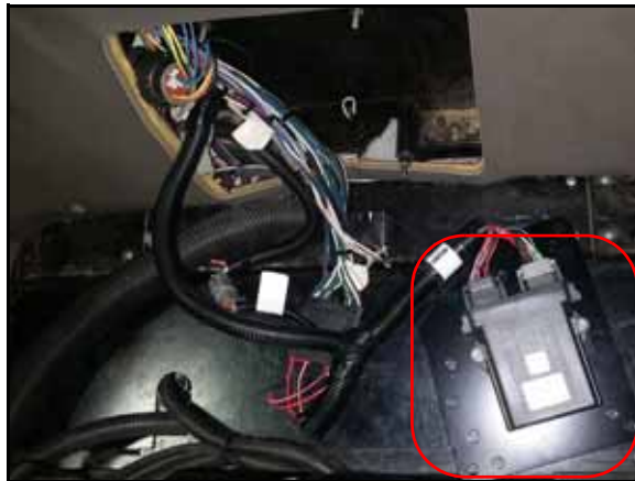
FIGURE 15. HDU Installed on HDU Mounting Bracket
