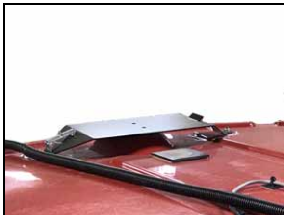
FIGURE 2. Machine's Existing Receiver Mounting Bracket
