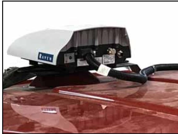
FIGURE 3. RS1 Unit Installed on Cab Roof
