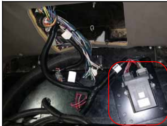
FIGURE 8. HDU Installed on HDU Mounting Bracket
