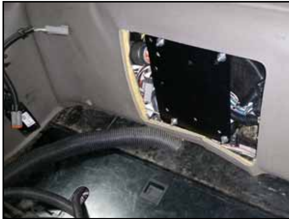
FIGURE 9. HDU Mounting Bracket Installed
