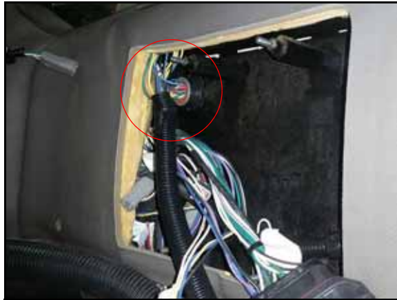
FIGURE 5. Machine's XB-7 Bulkhead Connection
