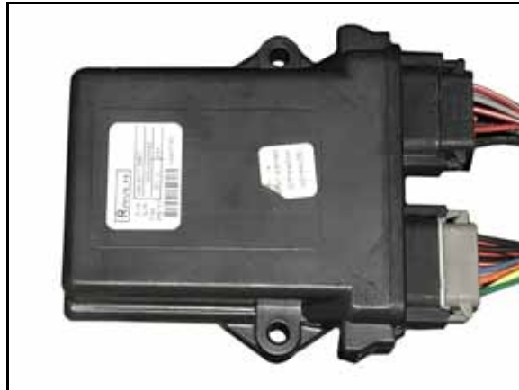
FIGURE 7. HDU Harness Cable Installed on HDU
