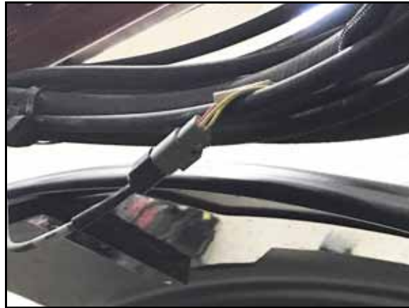
FIGURE 7. Machine's AutoSense Connection
