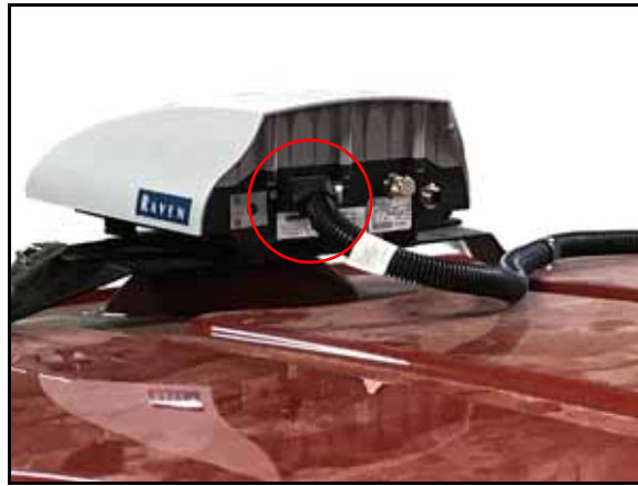
FIGURE 11. RS1 Tee Cable Connection
