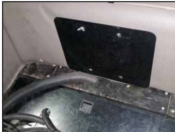
FIGURE 4. Access Panel to be Removed
