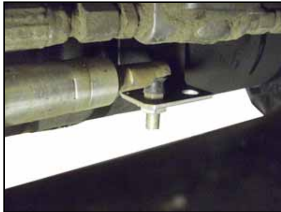
FIGURE 12. Base End Installed in the WAS Bracket
