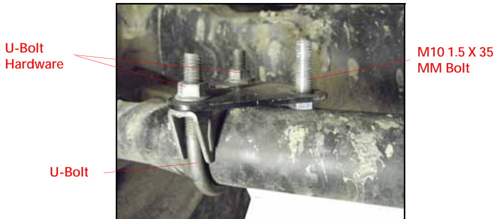
FIGURE 9. 4XXX Series WAS Mounting Bracket on Tie Rod
