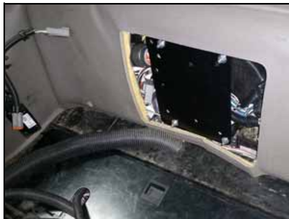
FIGURE 8. HDU Mounting Bracket Installed
