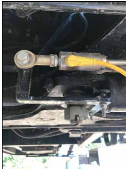
FIGURE 2. WAS Base End Mounting Brackets Installed
