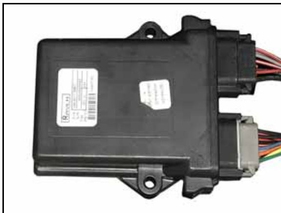
FIGURE 6. HDU Harness Cable Installed on HDU
