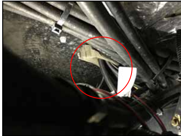
FIGURE 9. 12-Pin RS1 Harness Connector Routing
