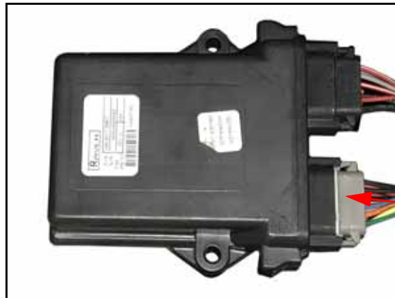
FIGURE 6. RS1 HDU Harness Cable Installed on HDU
