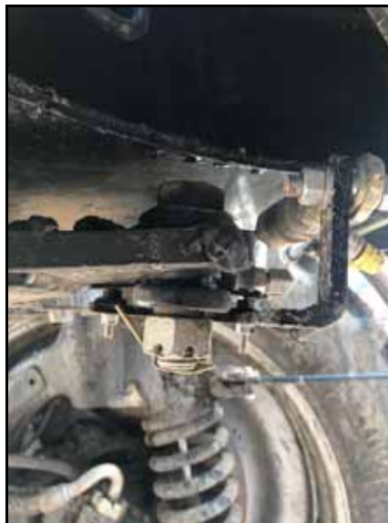
FIGURE 5. Base-End of WAS Installed on Base-End of Steering Cylinder
