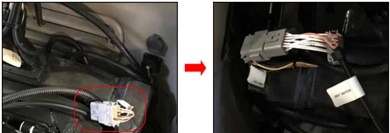
FIGURE 15. Seat Switch Harness Connections
