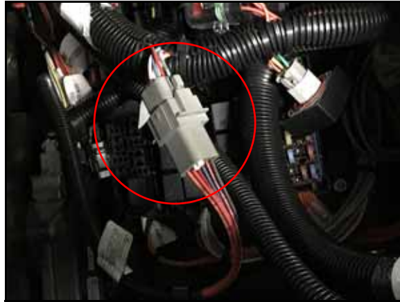
FIGURE 14. HDU Harness Cable Connection
