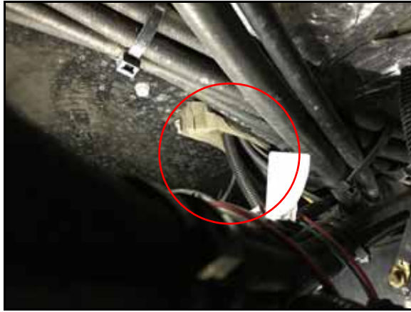
FIGURE 10. 12-Pin RS1 Harness Connector Routing
