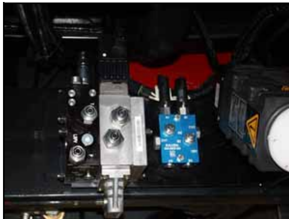
FIGURE 5. Steering Valve Installed on Mounting Bracket
