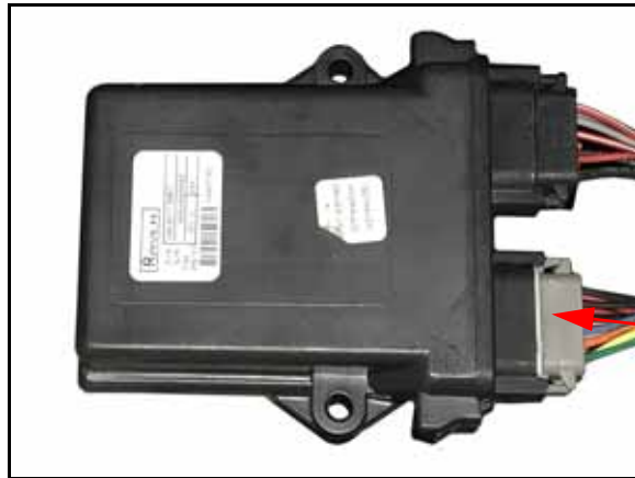
FIGURE 8. RS1 HDU Harness Cable Installed on HDU
