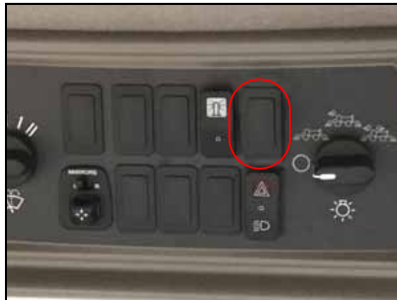
FIGURE 16. Master Switch Installation Location
