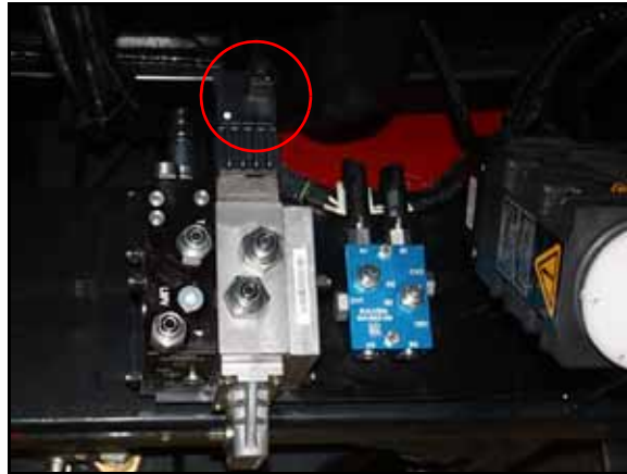
FIGURE 20. VALVE Harness Cable Installation Location
