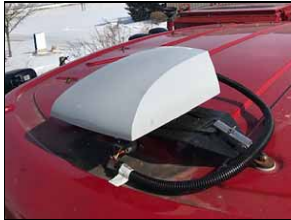
FIGURE 3. RS1 Unit Installed on Cab Roof
