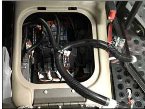
FIGURE 7. RS1 HDU Harness in Instructional Seat Compartment
