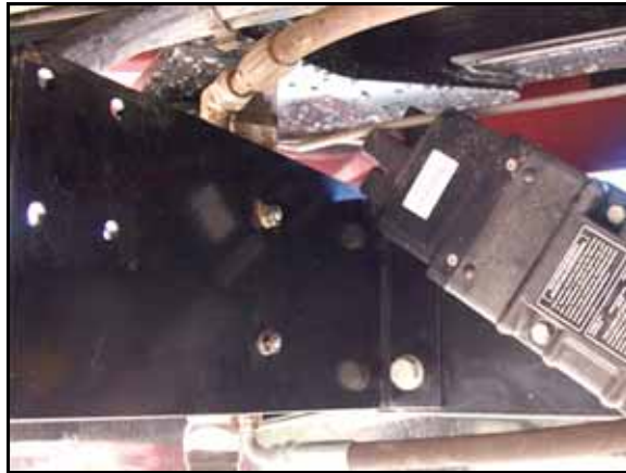
FIGURE 4. Mounting Bracket Installed
