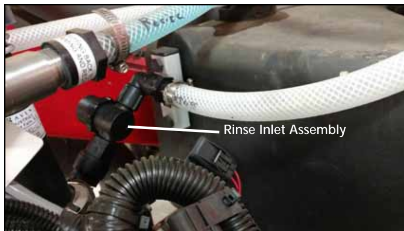
FIGURE 20. Rinse Inlet Assembly Attached to the Rinse Valve
