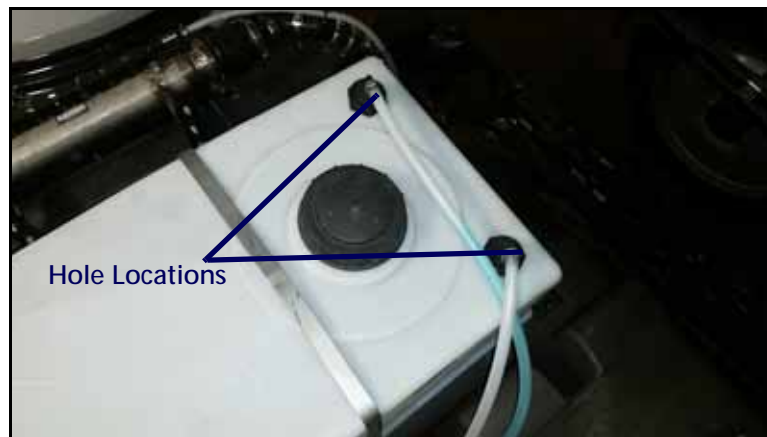
FIGURE 7. Holes on 56 Gallon Tank
