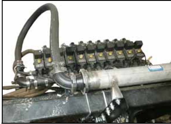
FIGURE 12. Mixer Outlet to Flowmeter Inlet Assembly
