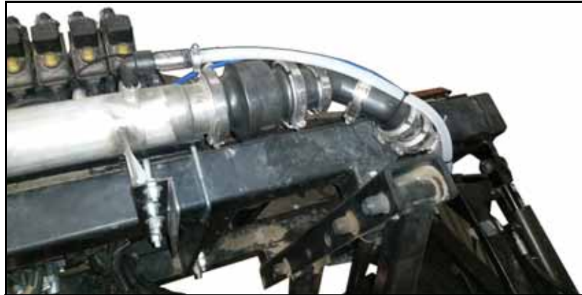
FIGURE 10. Carrier Hose to Elbow Installation
