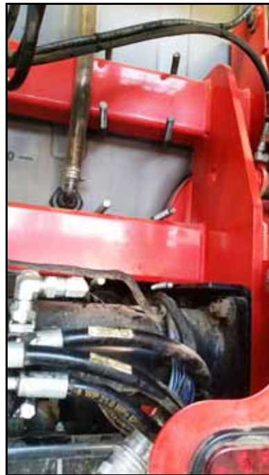
FIGURE 3. U-Tubes Installed Around Sprayer Frame
