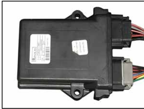
FIGURE 2. HDU Harness Cable Installed on HDU
