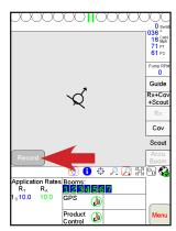
**Point, Group Of Points, Line**) can also be recorded, select the **Zone** button for a field boundary. On the *Record Field Feature* page, select *Field Boundary*, keep selection on *Auto Point Entry*, enter *Offset from center of swath* and direction of offset. An extended offset can be entered if the headlands are going to be filled in last. Select the **OK** button when finished.
