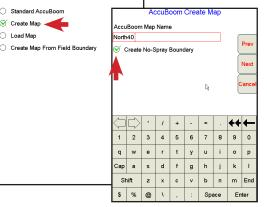
Map on the AccuBoom Setup page. Enter a name for the AccuBoom Map Name and keep selection for Create No-Spray Boundary. Continue with the rest of the job set up.
