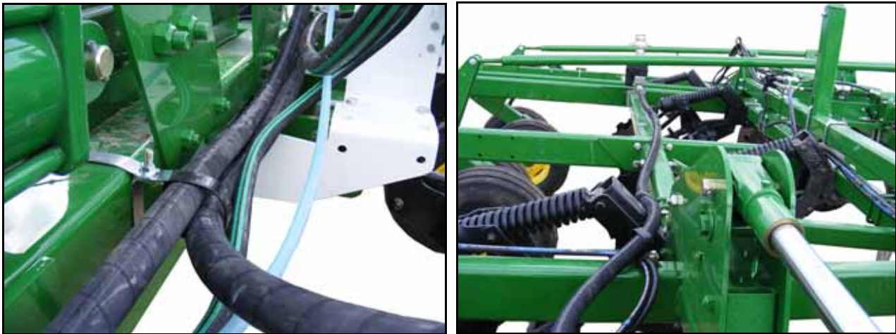
FIGURE 2. Acheminement du tuyau NH3
