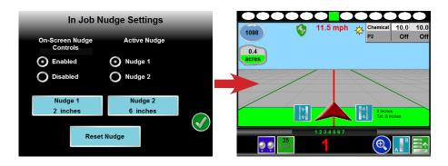
The on screen **Nudge** buttons for the active increment will be visible once a guidance line has been created.
