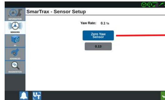
**Zero Yaw Sensor:** will clear the yaw reading to indicate no turning motion while sitting still. Normal range of the yaw sensor range is -2.0 to 2.0. Outside this range indicates a bad sensor in the steering node.
