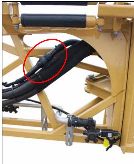
FIGURE 14. Primary and Secondary Boom Cable Connection at Mid-Boom Fold Point
