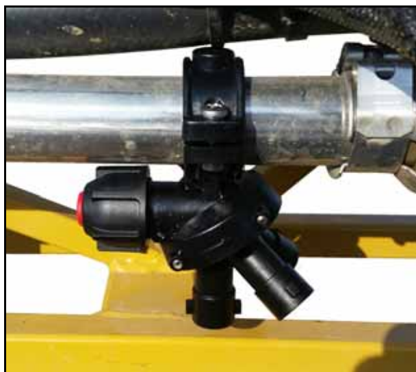
FIGURE 11. Triple Nozzle Body Installed
