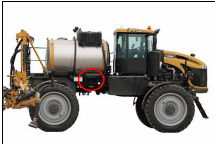
FIGURE 1. Chassis Cable Electrical Box Connection
