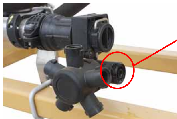
FIGURE 1. Nozzle Body Cap and Diaphragm Removed
