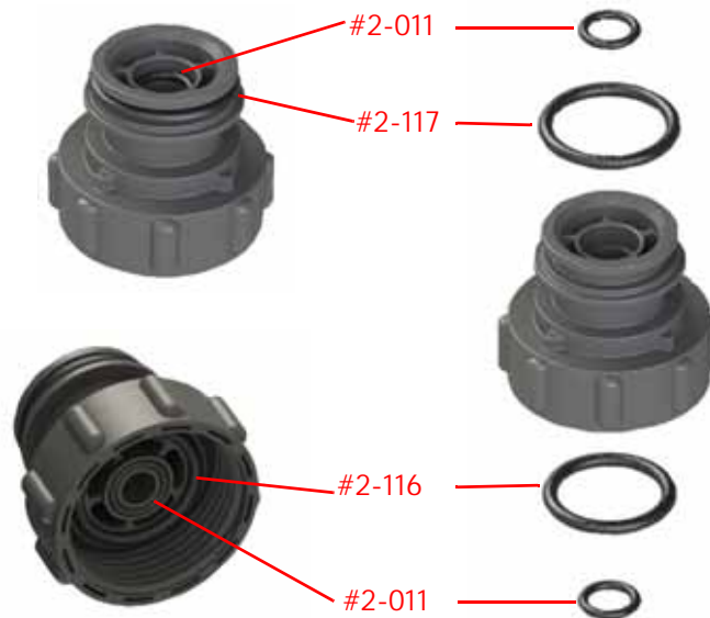
FIGURE 3. ProStop-E Adapter O-Ring Installation
