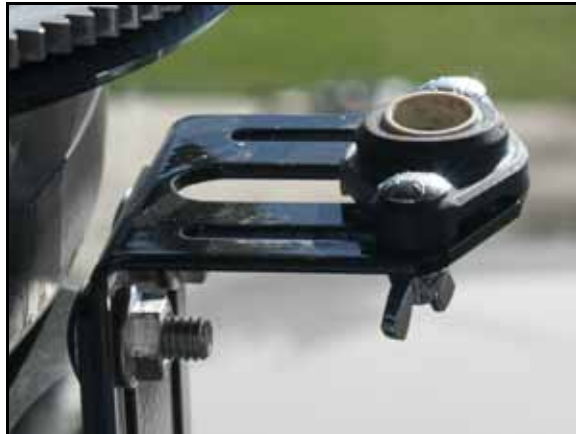
FIGURE 17. Flanged Bearing Assembly Installed
