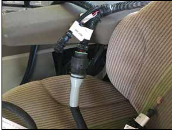
FIGURE 6. RS1 MD Connected to Console Cable
