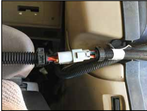
FIGURE 4. RS1 Tee Cable Connected to RS1 MD Cable
