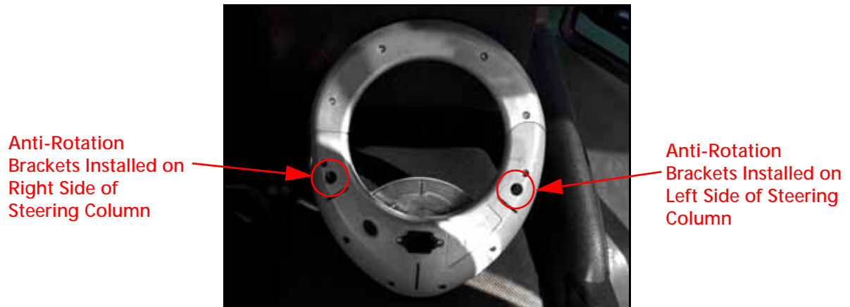
FIGURE 19. Anti-Rotation Pin Installation Locations
