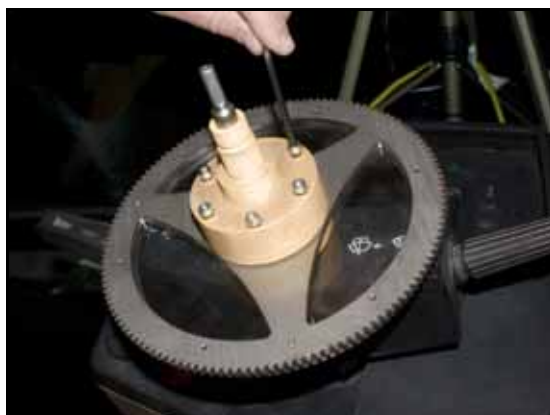
FIGURE 12. Spline Assembly Bolts Installed
