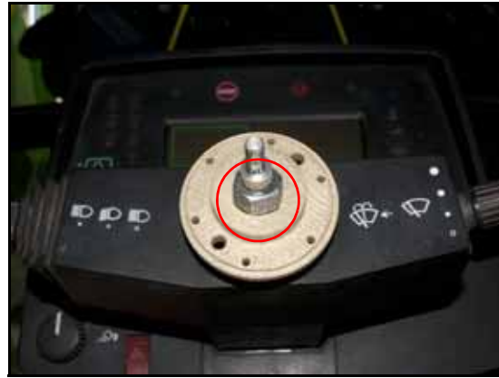
FIGURE 7. Machine's Steering Wheel Nut Installed
