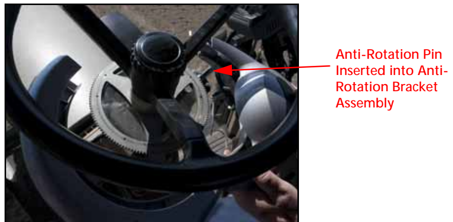
FIGURE 20. Anti-Rotation Pin Installed in Bracket Assembly
