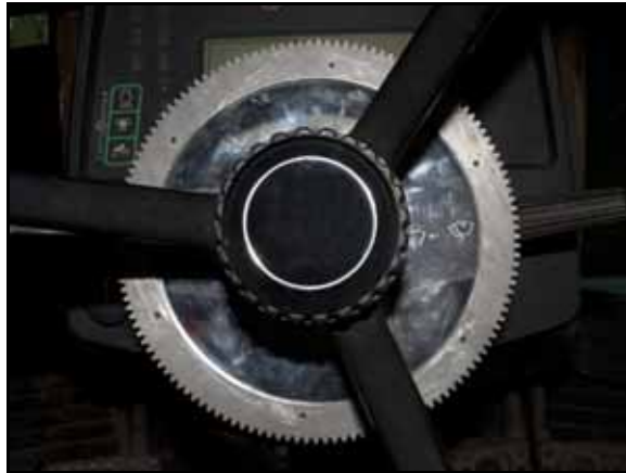
FIGURE 15. Steering Wheel Cap Reinstalled
