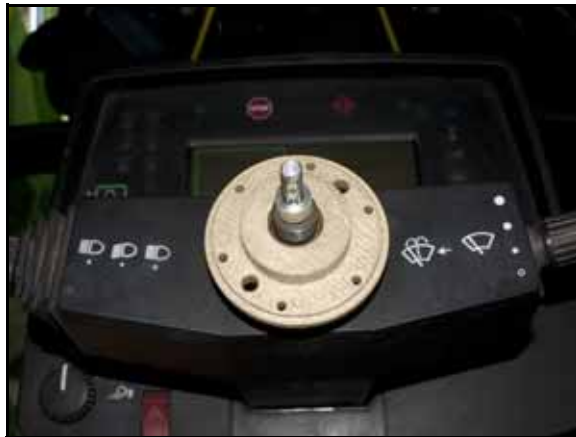
FIGURE 6. Female Spline Adapter Installed on Steering Column
