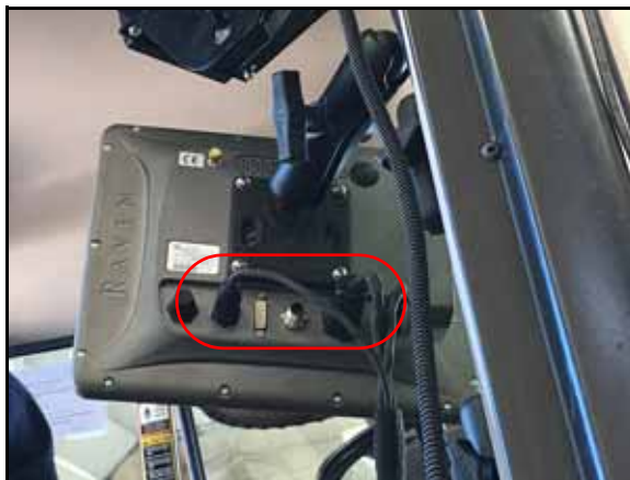
FIGURE 7. Console Cable Connected to Console
