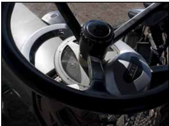
FIGURE 21. Mechanical Drive Installed
