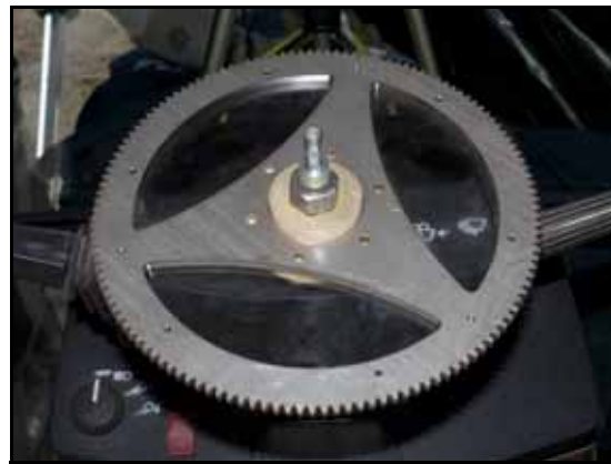
FIGURE 8. Ring Gear Assembly Installed
