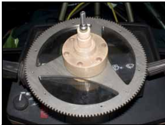
FIGURE 11. Male Spline Adapter Assembly Installed
