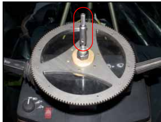
FIGURE 9. Telescope Adapter Assembly Installed (If Applicable)
