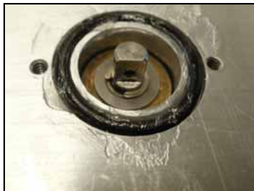
FIGURE 23. WAS with O-Ring and Di-Electric Grease Applied
