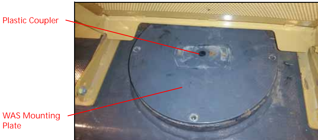
FIGURE 22. Plastic Coupler on WAS Mounting Plate
