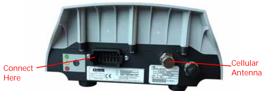
FIGURE 15. Cabling Connection on RS1 Unit
