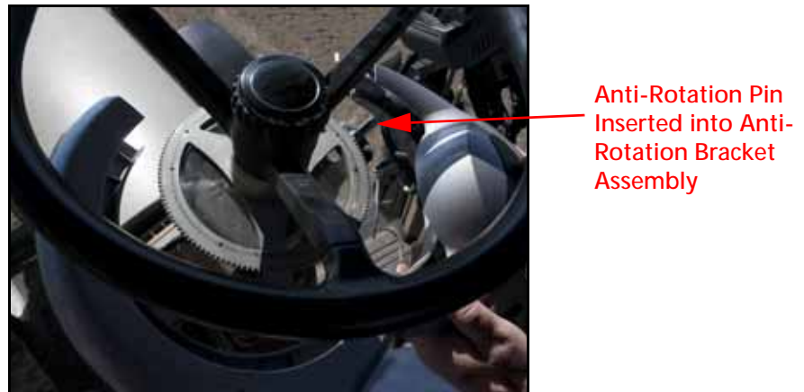
FIGURE 18. Anti-Rotation Pin Installed in Bracket Assembly
