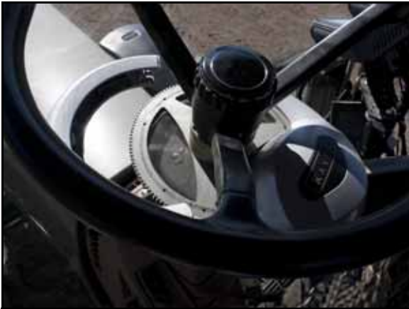
FIGURE 19. Mechanical Drive Installed
