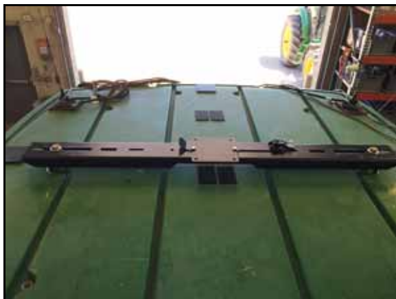
FIGURE 3. RS1 Crossbar Assembly Installed
