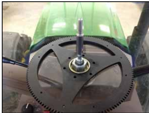
FIGURE 8. Ring Gear Assembly Installed
